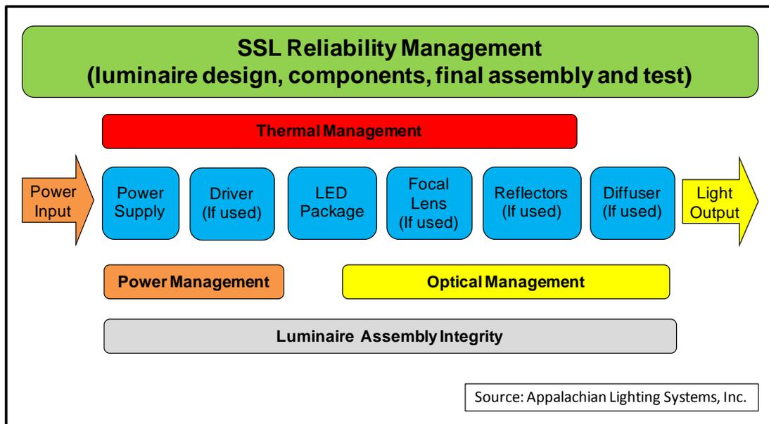
FIGURE 2. SSL LUMINAIRE COMPONENTS AND RELIABILITY CONSIDERATIONS
