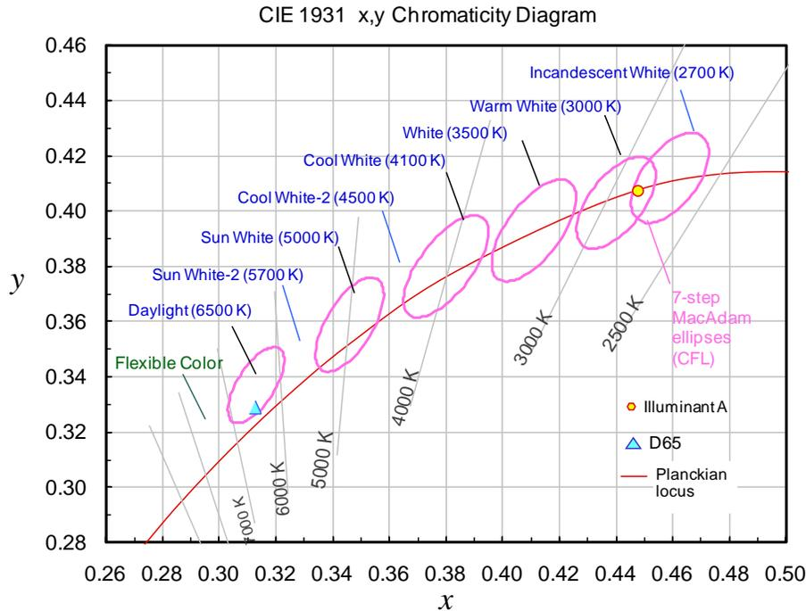
FIGURE 5. COLOR MATCHING TOLERANCES DEFINED IN TERMS OF 7-STEP MACADAM ELLIPSES CENTERED ALONG THE BLACK BODY CURVE. THE ELLIPSES SHOWN ARE DESIGNATED CCTs FOR CFLs.
