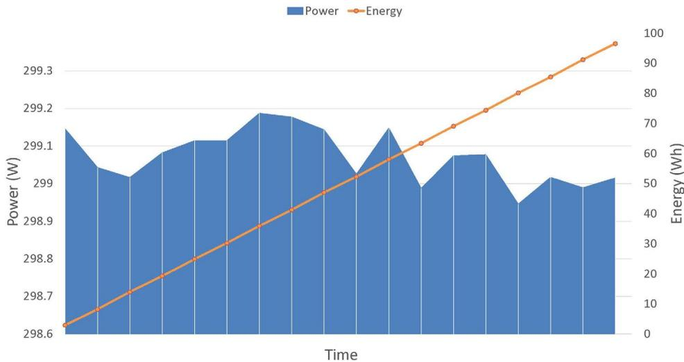
**Figure 6: Sample calculation of energy via the integration of power over time, using the trapezoidal rule.**
