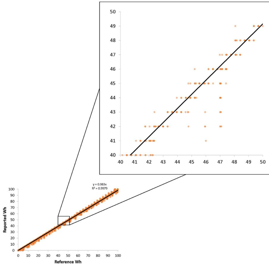
Figure 19: Example linear regression performed on the C3 reported energy data.
