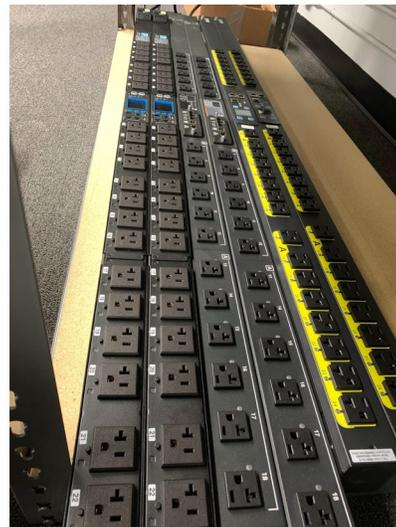
Figure 5: The three commercial-market, multiple-outlet PDUs that were tested (two units of each shown here).
