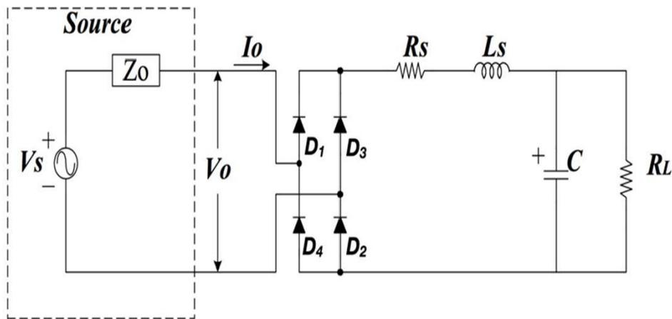
Figure A1. A rectified load equivalent circuit capable of drawing current with high harmonic content.
