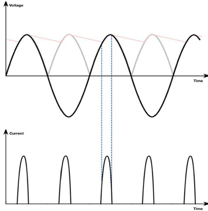
Figure A2. Example voltage and current waveforms for the rectified load.
