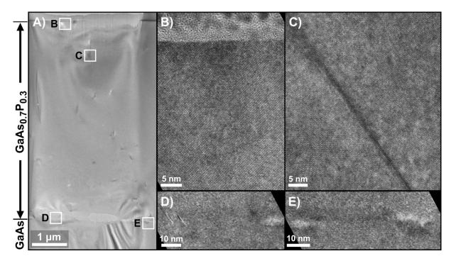
**Figure 23:** TEM of sample T10 FIB cross-section **A)** Overview of cross-section showing entire thickness of GaAs<sub>0.7</sub>P<sub>0.3</sub> film with few defects. The interface with the GaAs substrate is marked. **B)** HR-TEM of the surface showing no defects. **C)** HR-TEM of a dislocation. **D** and **E)** HR-TEM of interface showing no obvious threading dislocations and only few interfacial defects likely related to surface contamination.
