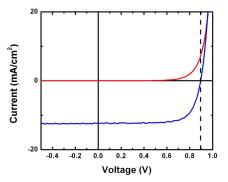
Figure 10: Light and dark IV curves for the 8.1% efficiency device from film 7.
