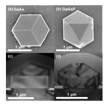
**Figure 31: A)** GaAs and **B)** GaAsP microstructure on GaAs (111) by selected-area epitaxy. **C)** and **D)** show cross-sectional TEM images prepared by FIB. The GaAs microstructures show twinning defects, while the GaAsP ones show a few interface dislocations due to the 1.3% lattice mismatch, but no twins.
