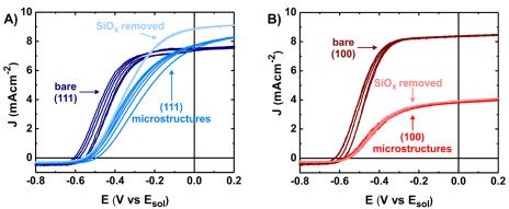
**Figure 30:** Representative illuminated JV curves for **A**) (111) and **B**) (100) microstructures. The (111) microstructures initially out-perform the bare (111) highly-doped substrate, and their performance is improved with removal of SiO<sub>x</sub>. Conversely, the performance of the (100) microstructures is far below the bare (100) highly doped substrate, and does not improve with etching of the dielectric.
