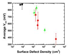
**Figure 14:** Average open-circuit voltage decreases with increasing absorber surface morphological defect density. Colors and marker shape indicate absorber films grown from different source pellets. Error bars show the standard deviation of the value for the 10 mesas fabricated from each *pn* junction. The data constitutes ~100 individual *pn* junction devices.
