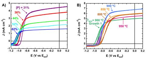
**Figure 24:** Representative JV curves. **A)** The decrease in  $J_{SC}$  across the composition series with increasing [P] is consistent with increasing  $E_g$  and the shift from direct to indirect  $E_g$ . **B)** The temperature series shows the best *J*-*E* characteristics for the samples grown at 900 °C; samples T3 and T5 have similar characteristics to T7 and therefore are omitted here. The compositional inhomogeneity of sample T1 (30.2%) appears to have reduced  $J_{SC}$ .
