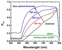
**Figure 11**:  $\phi_{int}$  at various etch depths of the device from film 4 with both emitter and absorber grown by CSVT.
