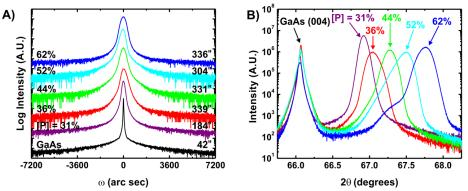
**Figure 19: A)** Rocking curve ( $\omega$ ) scans of each GaAs<sub>1-x</sub>P<sub>x</sub> (004) peak for the varied composition samples. FWHM values of all films are large compared to the GaAs substrate, a result of misfit dislocations. **B)**  $\theta/2\theta$  scans of the same samples, showing the shifting GaAs<sub>1-x</sub>P<sub>x</sub> (004) peak with increasing [P].
