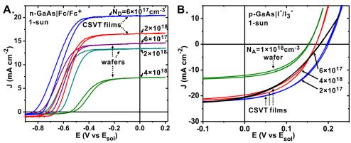
**Figure 4:** Photoelectrochemical *J-E* curves of (A) *n*-GaAs and (B) *p*-GaAs CSVT films and control wafers. The curves are labeled with the corresponding sample's free carrier concentration in cm<sup>-3</sup>. The selected curves are representative of other electrodes obtained from the same samples and from other samples with similar free carrier concentrations.
