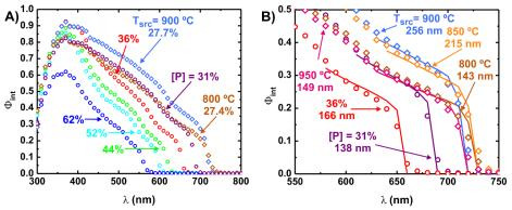
**Figure 25**:  $\phi_{int}$  data for **A**) the varied composition samples and select temperature series samples (T6 and T7) and **B**) at the band edge for representative samples of the temperature series (T2, 4, 6 and 7) and composition series samples C1 and C2. The Gärtner fits to the band edges are shown as solid lines.
