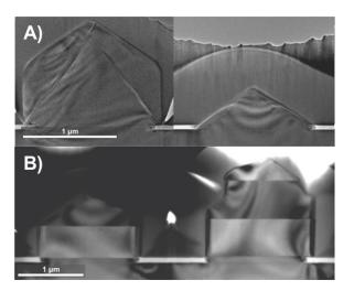
**Figure 29:** Cross-sectional TEM of **A)** (100) and **B)** (111)B GaAs microstructures. Note the stacks of defects present in the larger (100) microstructure which originate at the edge of the SiO<sub>x</sub> mask, and the single twin plane defects parallel to the growth surface in both (111)B microstructures.
