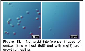
Huang et al. previously reported similar defect structures in CSVT GaAs, but they were unable to change the density of surface defects on non-miscut substrates.<sup>62</sup> In one trial, we found that a 5 minute anneal under H<sub>2</sub> (with [H<sub>2</sub>O] ~ 100 ppm) at 780 °C significantly improved the surface morphology of CSVT films grown on non-miscut wafers. This was not reproduced when a new Zn-doped pellet was used to grow thick films on wafers cleaved from the same ingot.
