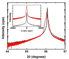
**Figure 26:** 20 XRD curve for showing the (004) reflection for an In<sub>1-x</sub>Ga<sub>x</sub>P film (red curve) which is nearly lattice-matched to the GaAs substrate (black curve). Inset: Rocking curves for the film and substrate (004) peaks.
