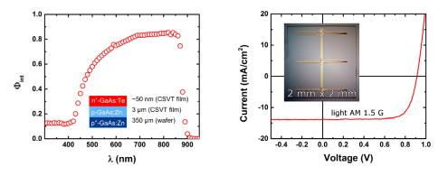
**Figure 15:** Left: JV curve for record efficiency device under 1-sun simulated illumination. Right: Internal quantum efficiency for the same device.
