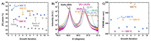
**Figure 20:** A) Evolution of [P] in the GaAs<sub>0.7</sub>P<sub>0.3</sub> source and the resulting varied temperature films. B)  $\theta/2\theta$  scans of the first seven varied temperature samples (the others are omitted for clarity). Note the compositional inhomogeneity in sample T1, [P] = 30.2%. C) FWHM values from rocking curve scans, which correlate strongly with growth temperature and film thickness. For A) and C), films grown at different  $T_{src}$  are indicated.
