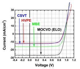
**Figure 16:** IV comparison of devices chosen for TPC/TPI study.
