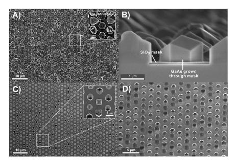
**Figure 27**: SEMs of microstructure growth. **A)** Plan-view and **B)** cross-section of (111)B microstructures with optimized growth conditions  $T_{src}$  = 850 °C,  $\Delta T$  = 10 °C for 10 min, 50 °C for 90 s **C)** Plan-view and **D)** 45° tilt of (100) microstructures with optimized growth conditions  $T_{src}$  = 850 °C,  $\Delta T$  = 30 °C for 10 min
