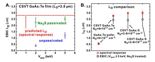
**Figure 7**: (A)  $L_D$  measured by EBIC on the same CSVT GaAs film before and after passivation by Na<sub>2</sub>S. The dashed line indicates the  $L_D$  predicted by spectral response. (B) Comparison of  $L_D$  obtained by spectral response and EBIC techniques.
