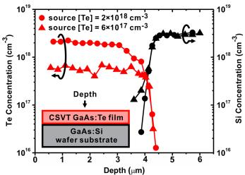
**Figure 2:** SIMS depth profiles of two *n*-GaAs films grown from differently-doped GaAs:Te sources on GaAs:Si substrates. The Te depth profiles are shown in red and Si in black. Circles denote the film was grown from a source containing [Te] =  $2 \times 10^{18}$  cm<sup>-3</sup>, triangles denote the film was grown from a source with [Te] =  $6 \times 10^{17}$  cm<sup>-3</sup>.
