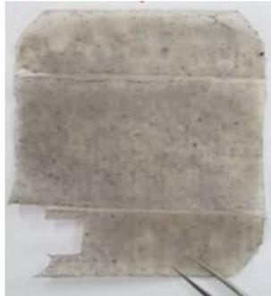
Photo of EVA sample separated from glass for no delamination portion.
