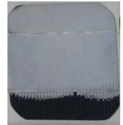
2. Separate an EVA sheet backside of a cell
