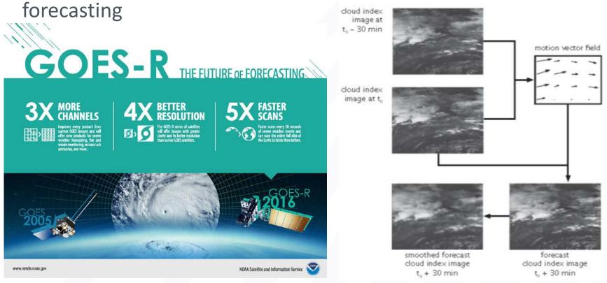
Images from *newest satellite platform GOES-R* will be utilized to generate higher resolution solar forecast data.
