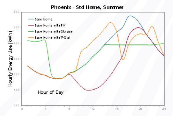
Assumed 3.6 kW PV, 4.4 kW/7.7 kWh storage with algorithmic control of load shapes for storage and Tstat technologies.
