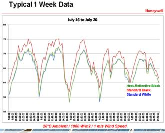
Typical daily and weekly comparisons of 3 independent grid-connected module arrays illustrating that the backsheet employed can impact NMOT. Note that the module with the "heat-reflective" black backsheet displays average operating temperatures closer to those of a typical white module.
