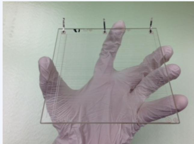
**Dielectric stop-gap printed over one phase**      **Finished EDS fabricated with screenprinting**
