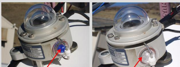
Cartridge filled with desiccant SiO<sub>2</sub>
