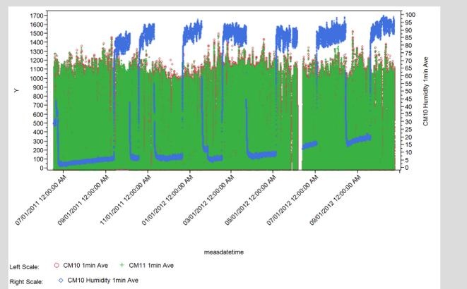
By swapping salt and desiccant, periods of high & low humidity are alternated so as not to destroy pyranometer
