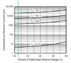
Typical Reverse Leakage Characteristics
