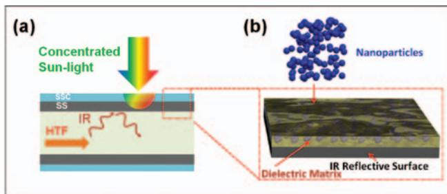
Schematic of the proposed spectral selective coating (SSC). The illustration on the left shows how concentrated sunlight is absorbed by the SSC layer on a stainless steel tube to raise the temperature of the heat transfer fluid. On the right, the SSC with nanoparticles is embedded in a dielectric matrix. *Illustration from University of California San Diego*
