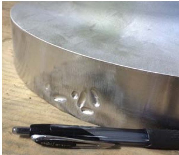
Figure 3-3. Surface Defect in the Exhaust Reducer Housing
