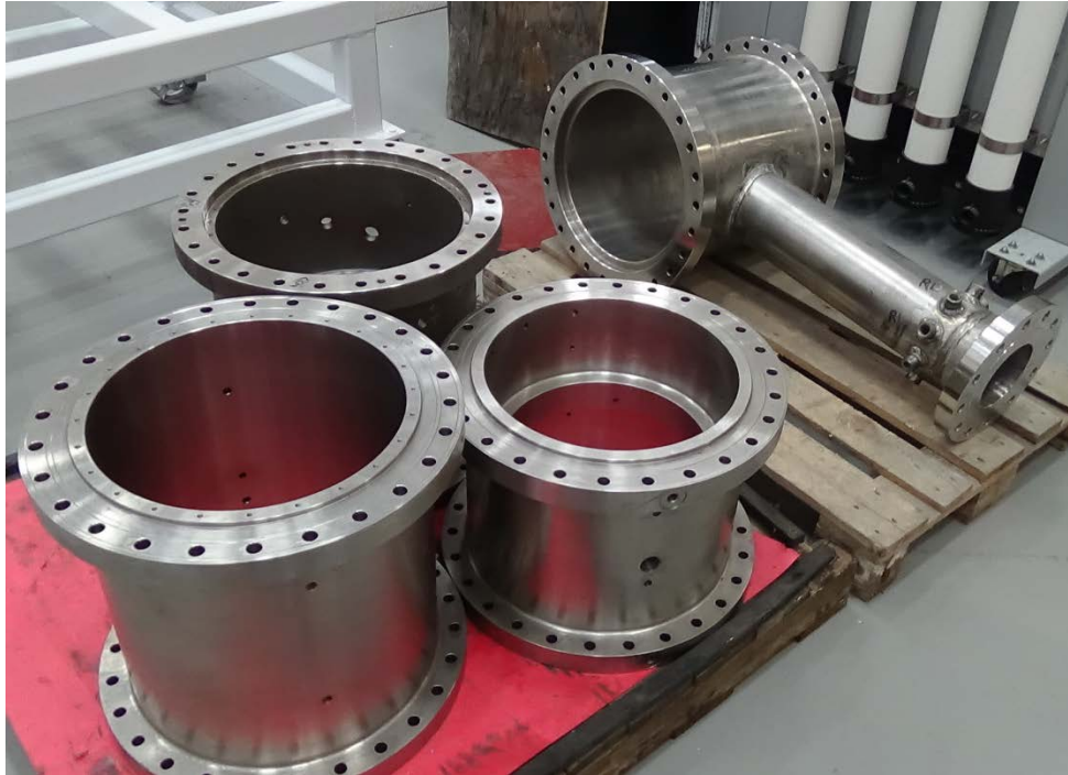
Figure 3-6. Combustor Housings after Final Machining
