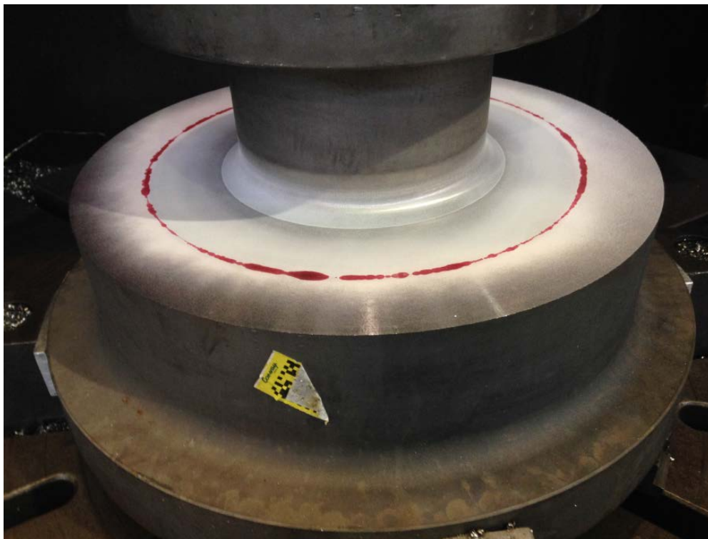
Figure 3-5. Exhaust Reducer Housing after Electron Beam Weld, before Final Machining
