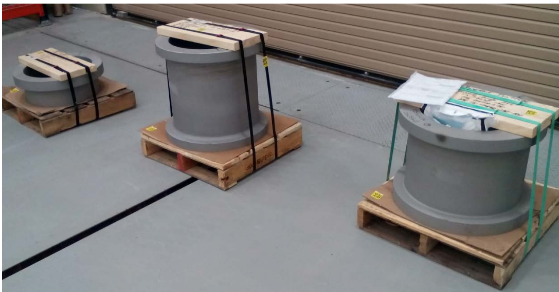
Figure 3-2. Spin-Cast Casings Before Final Machining
