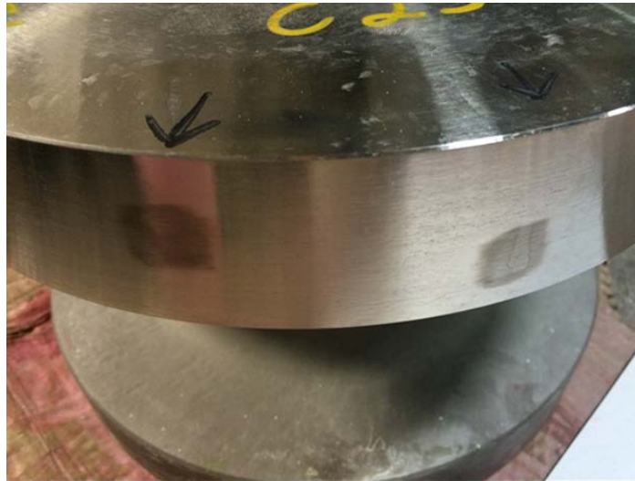
Figure 3-4. Weld Repair of Exhaust Reducer Housing Defect
