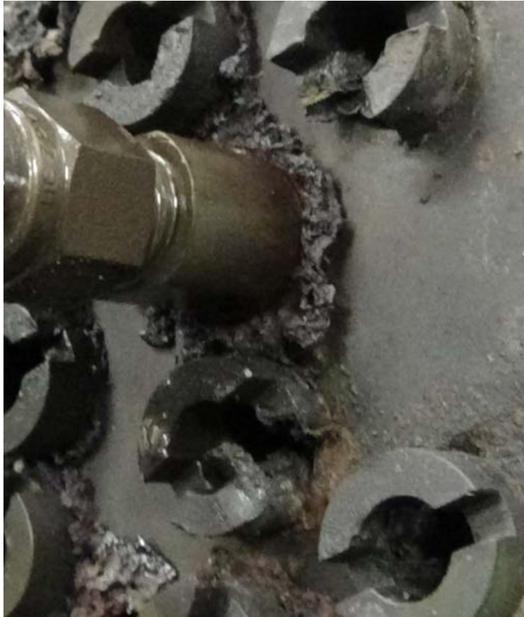
Figure 4-3. Evidence of Combustion on the Upstream Side of the Injector
