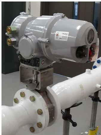
Figure 3-14. Rotork Four Inch Diameter Back-Pressure Control Valve
