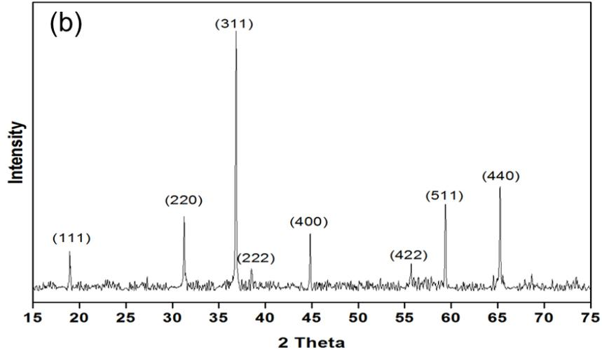
**Fig. 3.** X-ray diffraction pattern of Co oxide powders after stabilizing at 750°C for 2 hours, showing the Co<sub>3</sub>O<sub>4</sub> phase.
