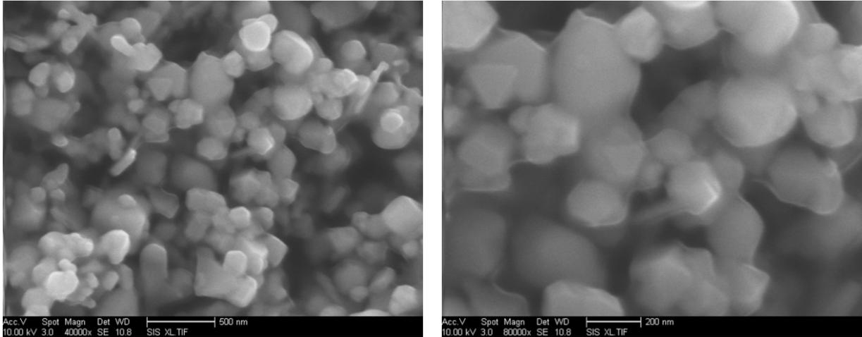
**Fig. 7.** Copper iron manganese ( $\text{CuFeMnO}_4$ ) particles observed with SEM have particle size of 100-300 nm.
