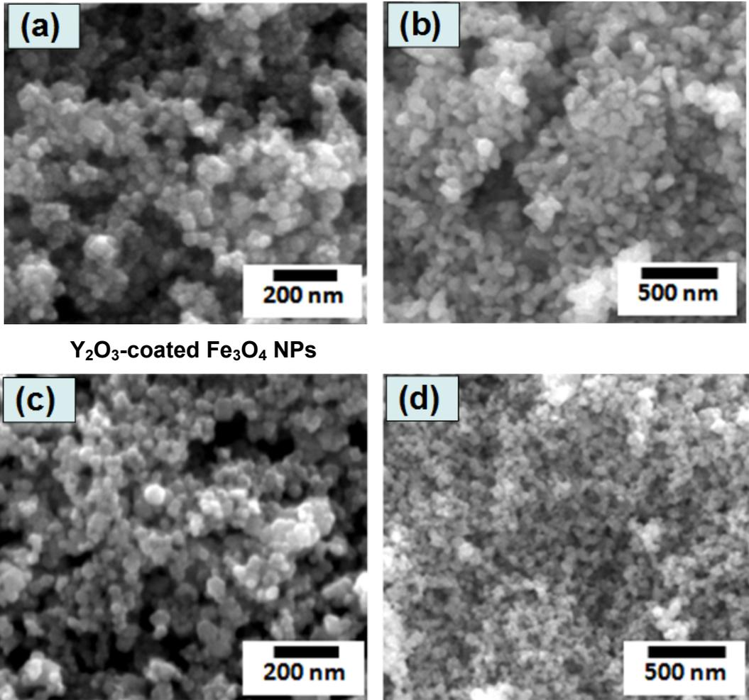
**Fig. 12.** SEM images showing the size change of bare Fe<sub>3</sub>O<sub>4</sub> and Y<sub>2</sub>O<sub>3</sub>-coated Fe<sub>3</sub>O<sub>4</sub> NPs depending on the annealing temperature. (a)~(b) : Fe<sub>3</sub>O<sub>4</sub>, (c)~(d) : Y<sub>2</sub>O<sub>3</sub>-coated Fe<sub>3</sub>O<sub>4</sub>, (a) and (c) : As-made, (b) and (d) : annealed at 750 °C for 2 hr.
