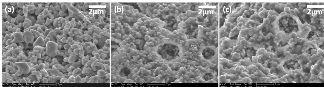
**Fig. 14.** SEM images of the porous  $\text{Co}_3\text{O}_4$  layers employing the polymer with the polymer beads of volume ratio 1:2 and 1:3 were shown in (a)-(c), respectively.
