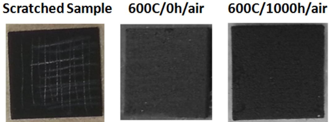
**Fig. 30.** Photos for (left) an impaired CuFeMnO<sub>4</sub>/CuCr<sub>2</sub>O<sub>4</sub> sample by scratching, (middle) a repaired sample by new spray coating on the scratched surface, and (right) a repaired sample after isothermal test.
