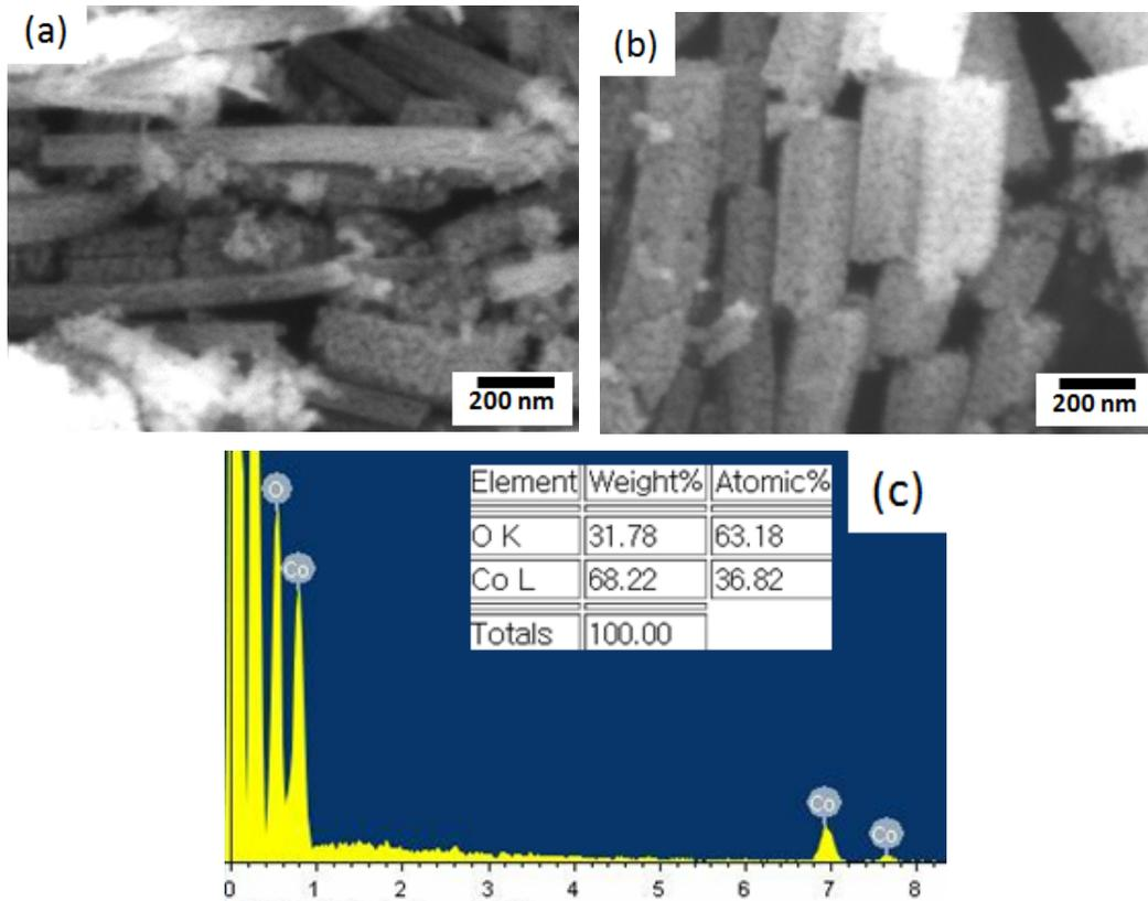
**Fig.4.** SEM images showing cobalt oxide ( $\text{Co}_3\text{O}_4$ ) nanorods ; (a) long nanorods with high aspect ratio and (b) short nanorods with low aspect ratio. And (c) EDX analysis result.
