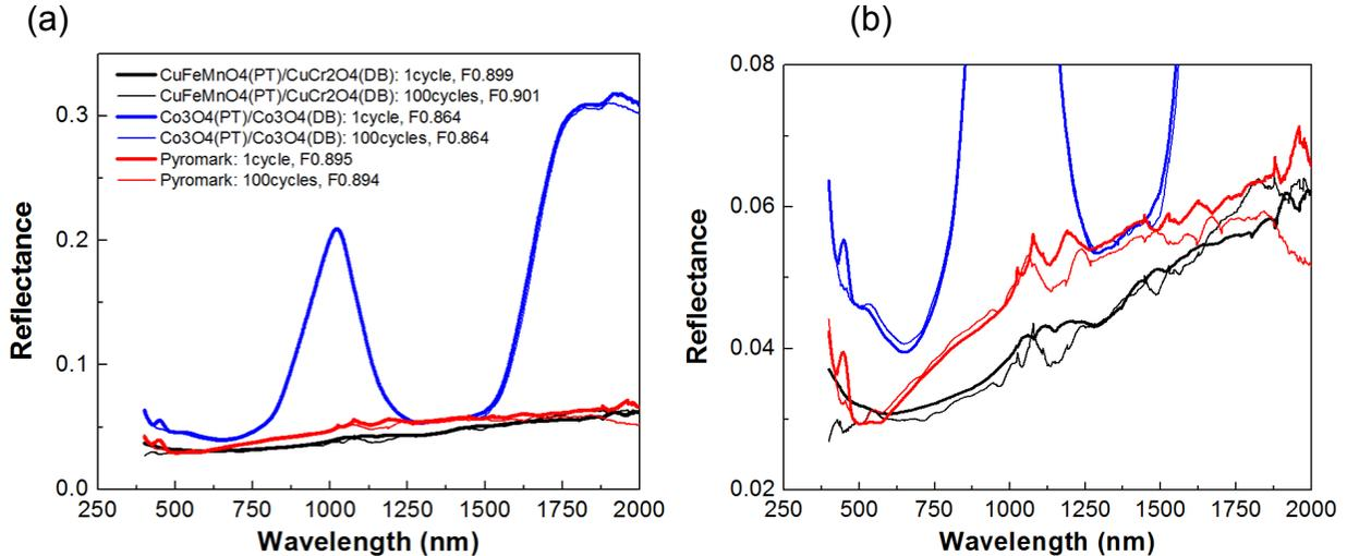
**Fig. 20.** Comparison of reflectance and FOM between 1-cycled samples and 100-cycled samples from RT to 600°C in air. (PT: porous top layer, DB: dense bottom layer)
