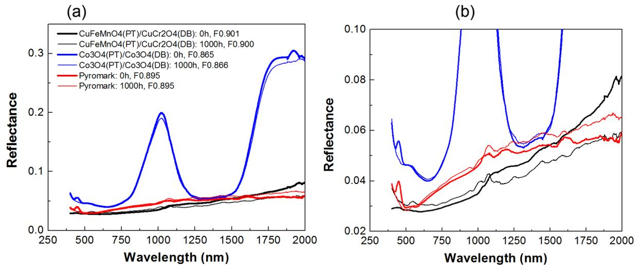
**Fig. 21.** Comparison of reflectance and FOM between as-prepared samples (0h) and samples annealed at 600°C/1000h/air. (PT: porous top layer, DB: dense bottom layer)
