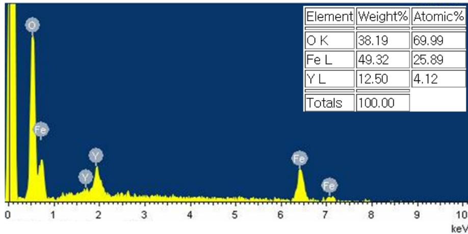
**Fig. 11.** EDX analysis result of Fe<sub>3</sub>O<sub>4</sub>-Y<sub>2</sub>O<sub>3</sub> core-shell nanoparticles.
