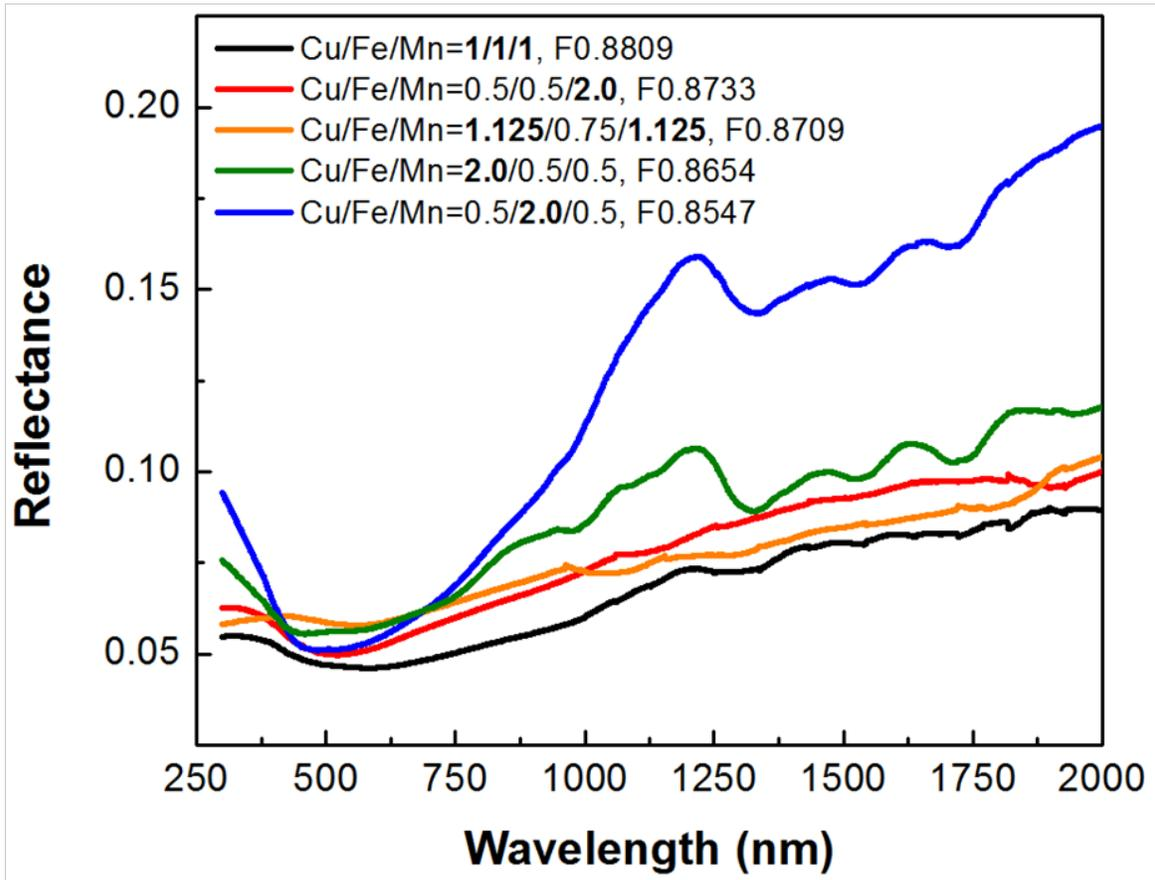
**Fig. 8.** Reflectance of SSC layers made of copper iron manganese particles with different atomic ratio (Cu/Fe/Mn). All samples had a dense single layer and were annealed with the condition of 750 °C/2h/air before reflectance measurement.
