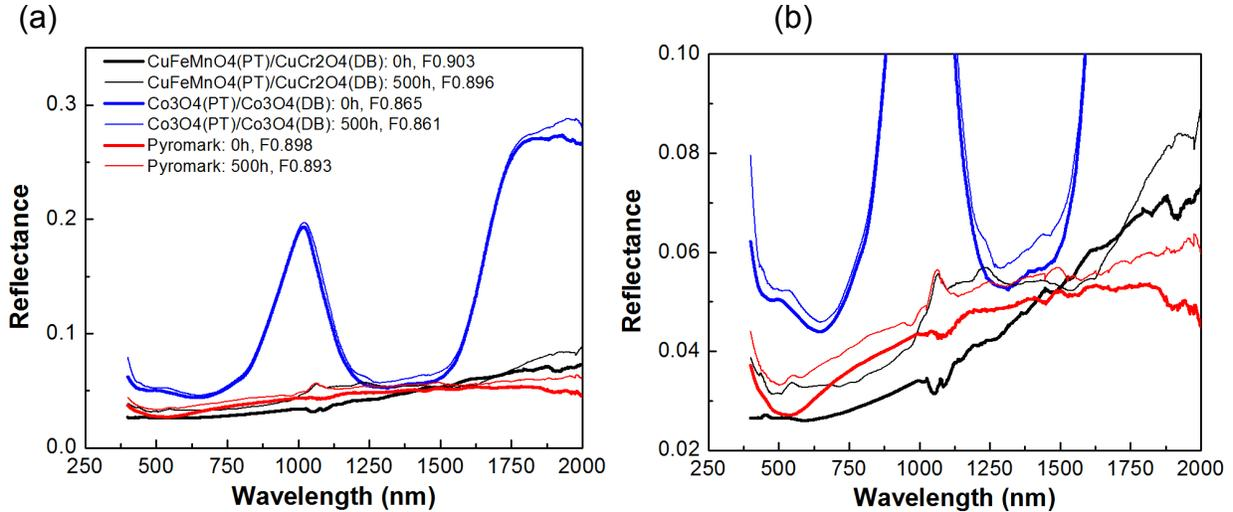
**Fig. 26.** Comparison of reflectance and FOM between as-prepared samples (0h) and samples annealed at 750°C/500h/air. (PT: porous top layer, DB: dense bottom layer)
