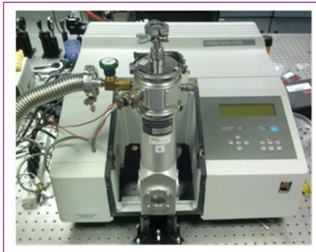
**Fig. 18.** High temperature stage integration into Mattson® based FTIR system.
