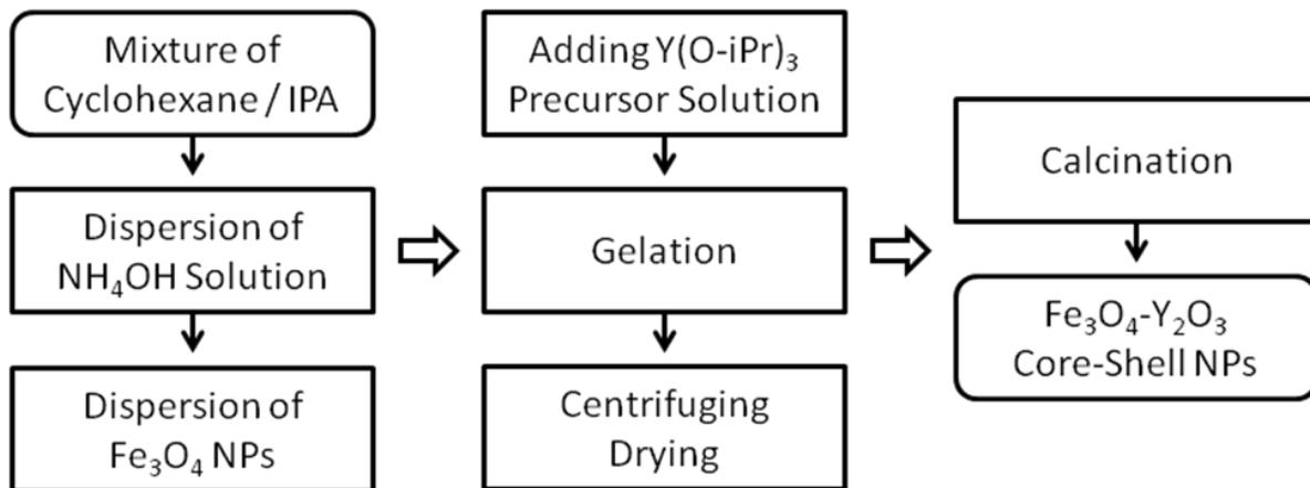
**Fig. 9.** The nano-shell synthesis procedure to make  $Fe_3O_4$ - $Y_2O_3$  core-shell NPs.
