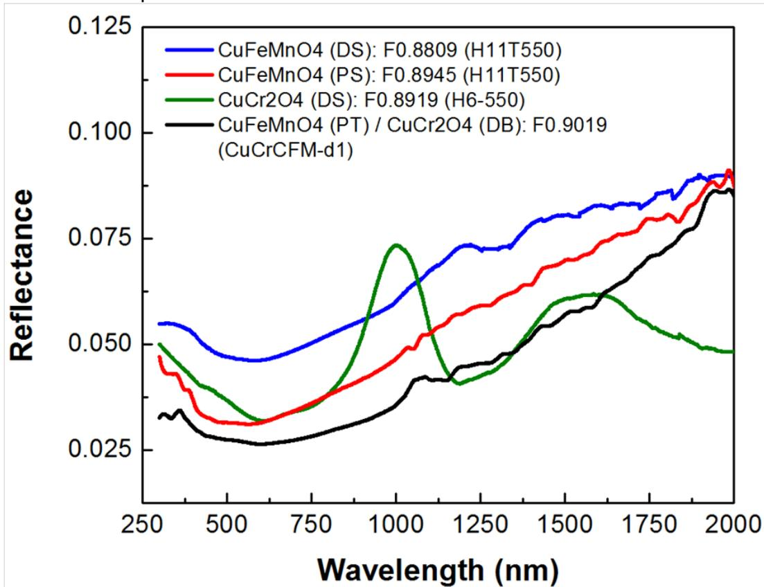
**Fig. 16.** Effect of porous layer structure and double layer on reflectance for SSC layers made of copper chromite particles and copper iron manganese particles. DS: dense single layer, PS: porous single layer, PT: porous top layer, and DB: dense bottom layer.
