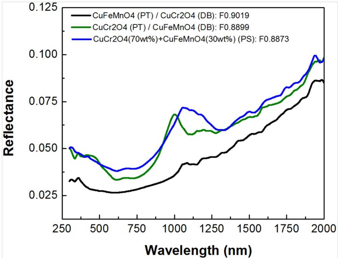
**Fig. 15.** Reflectance of double-layered sample and a single composite layered samples, fabricated with copper chromite and copper iron manganese oxide nanoparticles. All samples were annealed with the condition of  $750\text{ }^\circ\text{C}/2\text{h}/\text{air}$  before measuring. **PT**: porous top layer, **DB**: dense bottom layer, and **PS**: porous single layer.
