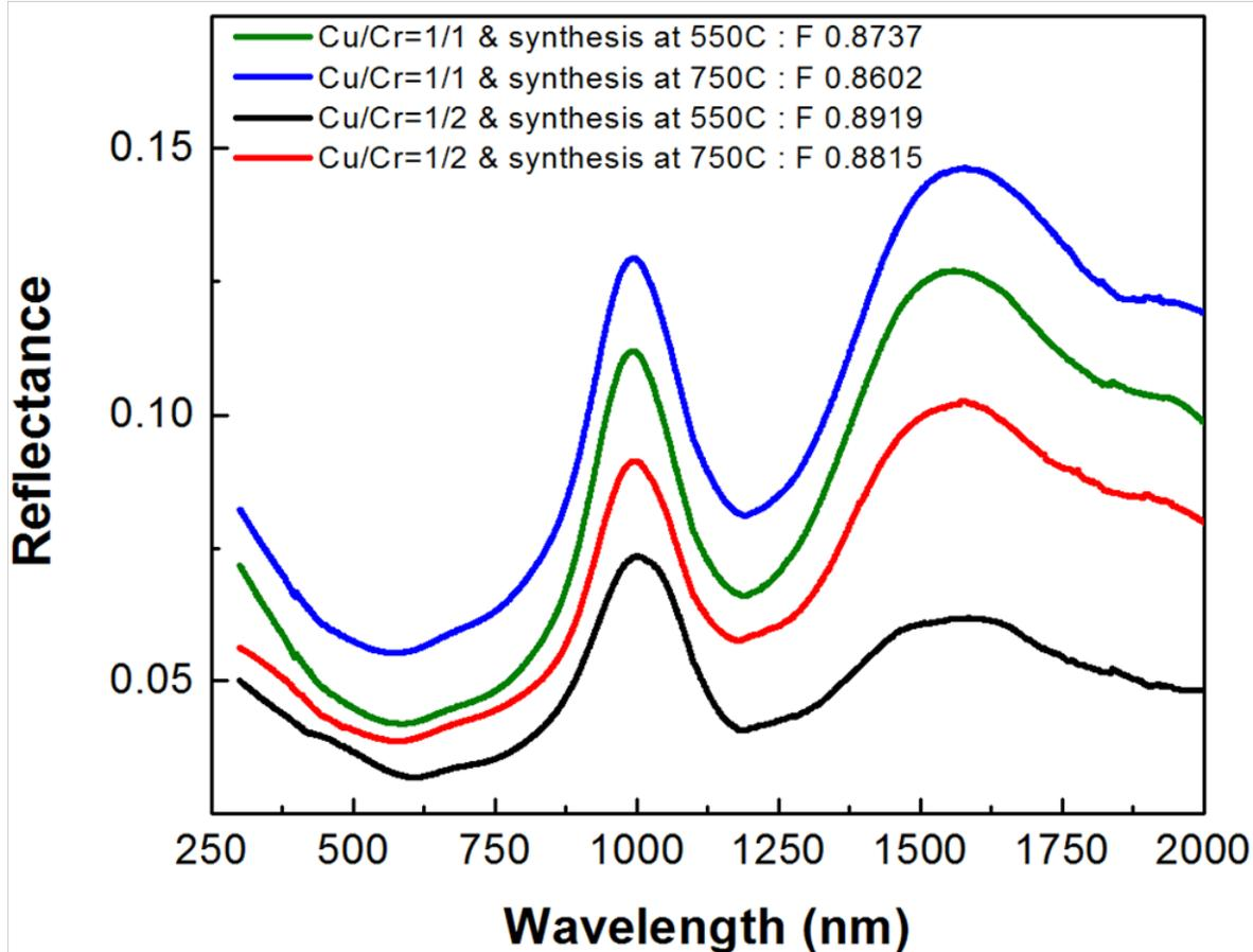
**Fig.6.** Reflectance change of SSC layers made of copper chromite nanoparticles with different atomic ratio (Cu/Cr) and crystallized at different temperatures. All coated samples were annealed with conditions of 750 °C/2h/air before reflectance measurement.
