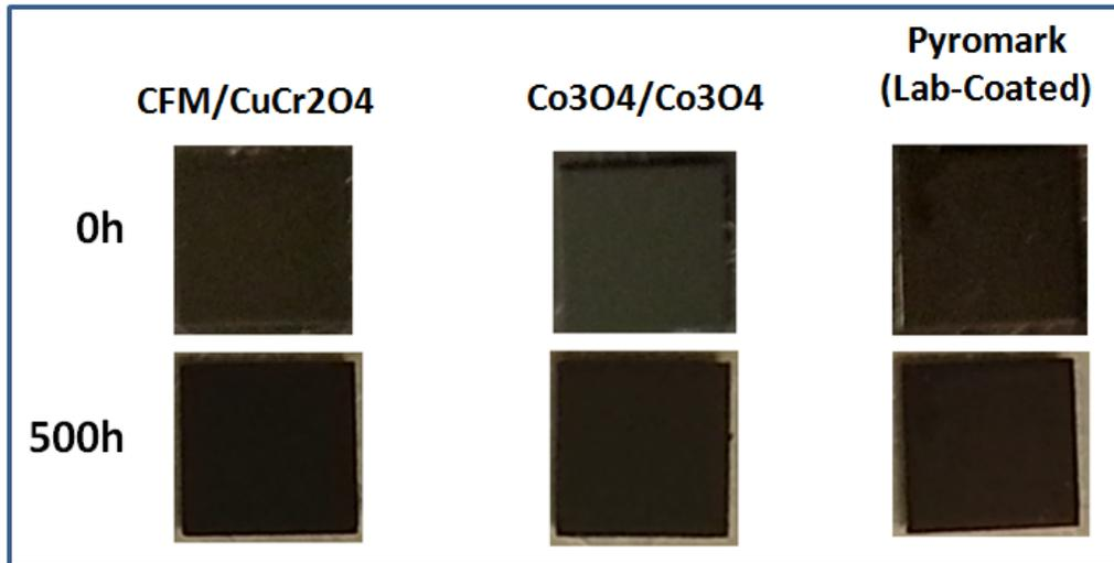
**Fig. 29.** Photos of samples taken before (0h) and after isothermal test (750°C/500h/air).
