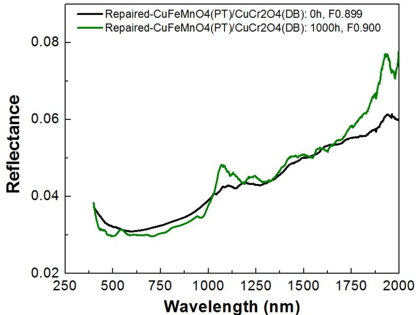
**Fig. 31.** Reflectance and FOM comparison between as-repaired CuFeMnO<sub>4</sub>/CuCr<sub>2</sub>O<sub>4</sub> (0h) and annealed one (600°C/1000h/air).
