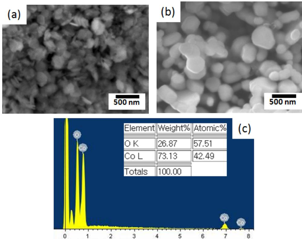
**Fig.2.** SEM images showing cobalt oxide nanoparticles (a) as-synthesized and (b) after annealing at 750  $^\circ\text{C}$  for 2 hr, and (c) EDX analysis results.
