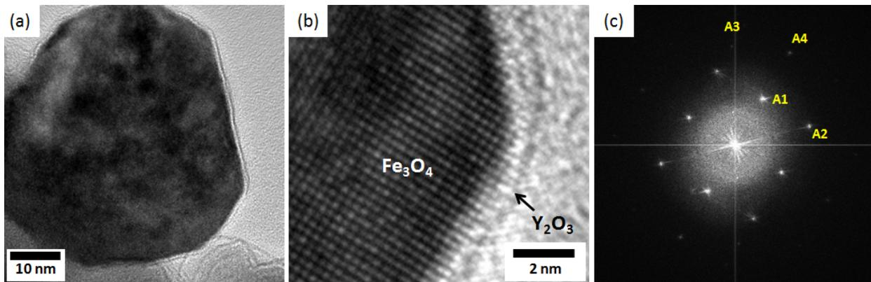
**Fig. 10.** (a) TEM images of  $Fe_3O_4$ - $Y_2O_3$  core-shell nanoparticles, (b) its magnified lattice image, and (c) its FFT patterns for the image (b).
