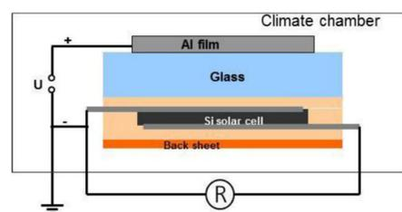
Fig. 4: Scheme of experimental setup 1
