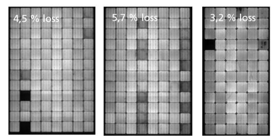
Fig. 9: Example where a few degraded cells with arbitrary distribution lead to rel. high performance loss (8 A)
