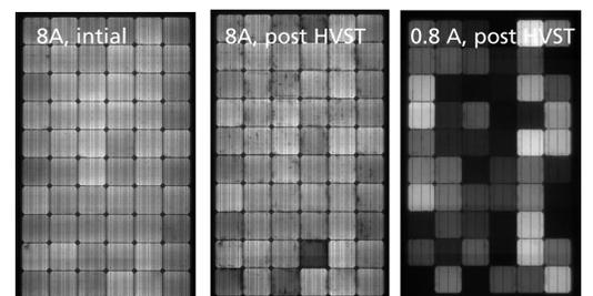
Fig. 11: Local shunting of solar cells leads to cloudy EL image of cells (here: power loss 15 %)
