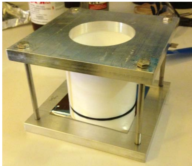
Attachment of reactor fixture for application of SAM to substrate
