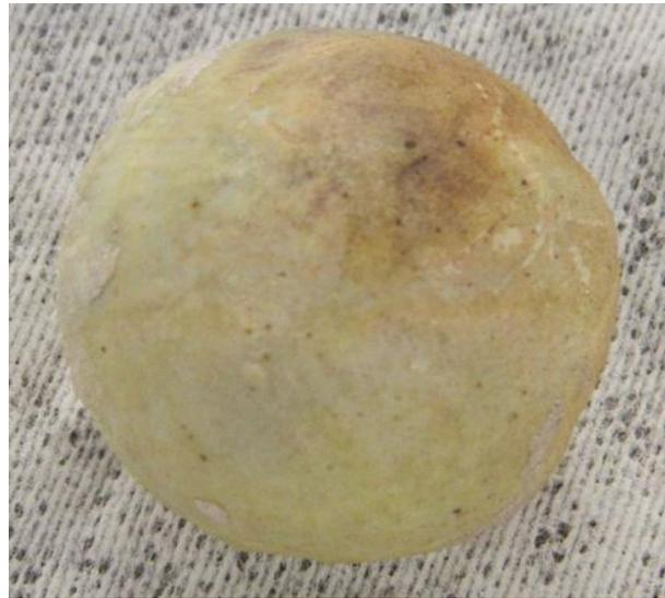
Intact salt capsule after thermal testing
