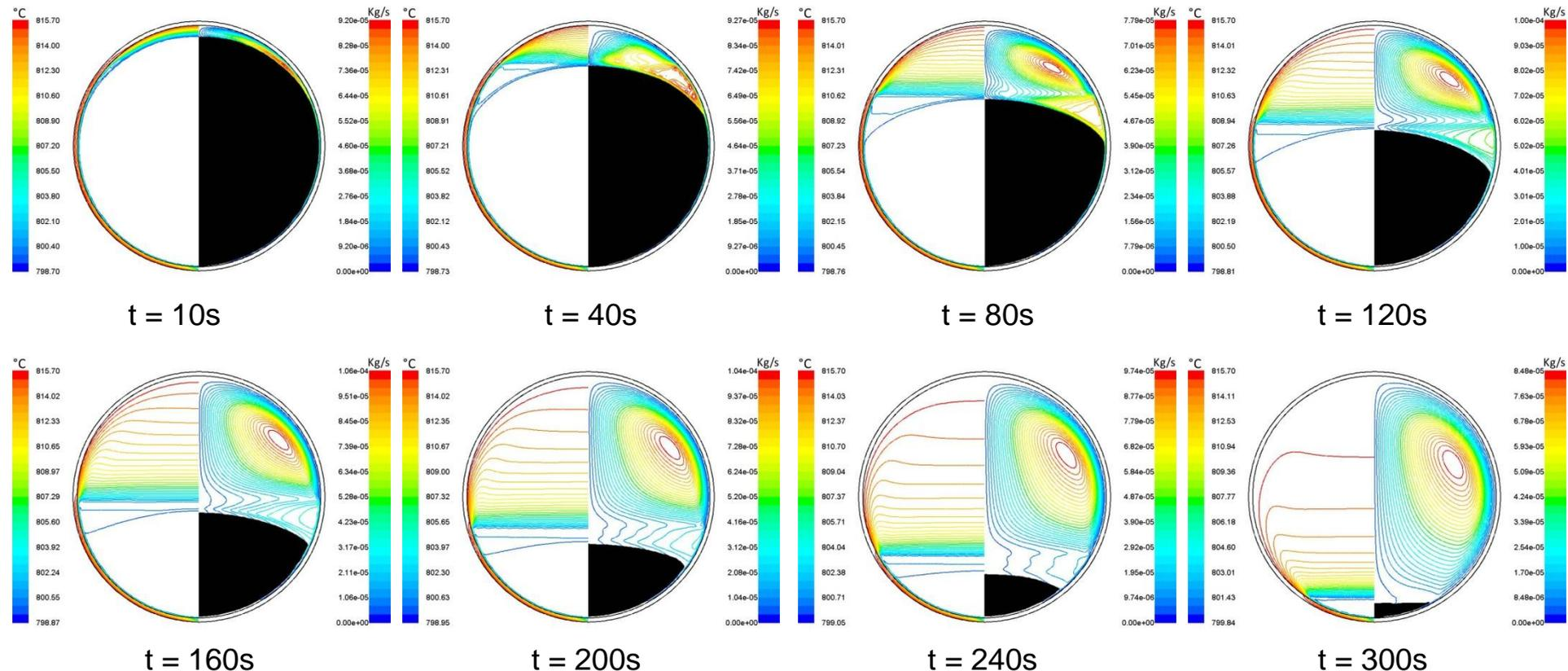
Fig. 2 Predicted evolution of the solid fraction, isotherms and streamline contours.
