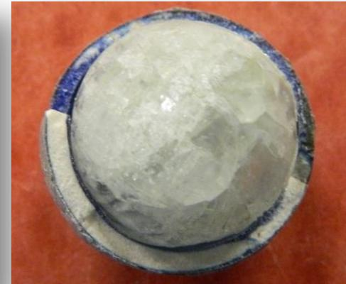
The pellet was cut open to check the diffusion of the salt into the ceramic layer
