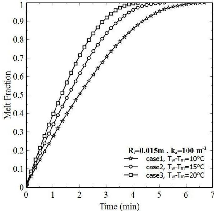
Fig. 3 Effect of the outer temperature.
