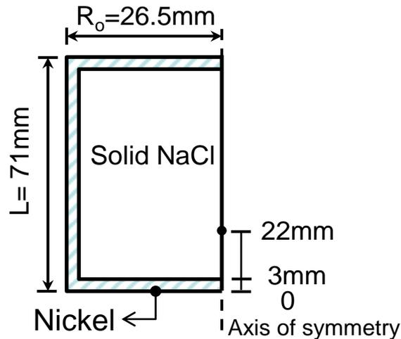
Fig. 7. Schematic of the system.
