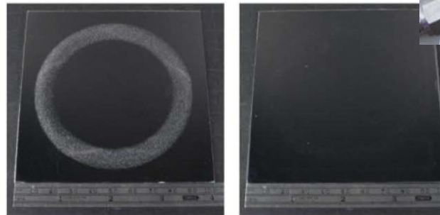
Fig 4. Taber abrader damage to polymer film reflector sample without ARC coating (left) and almost no damage with ARC coating (right).
