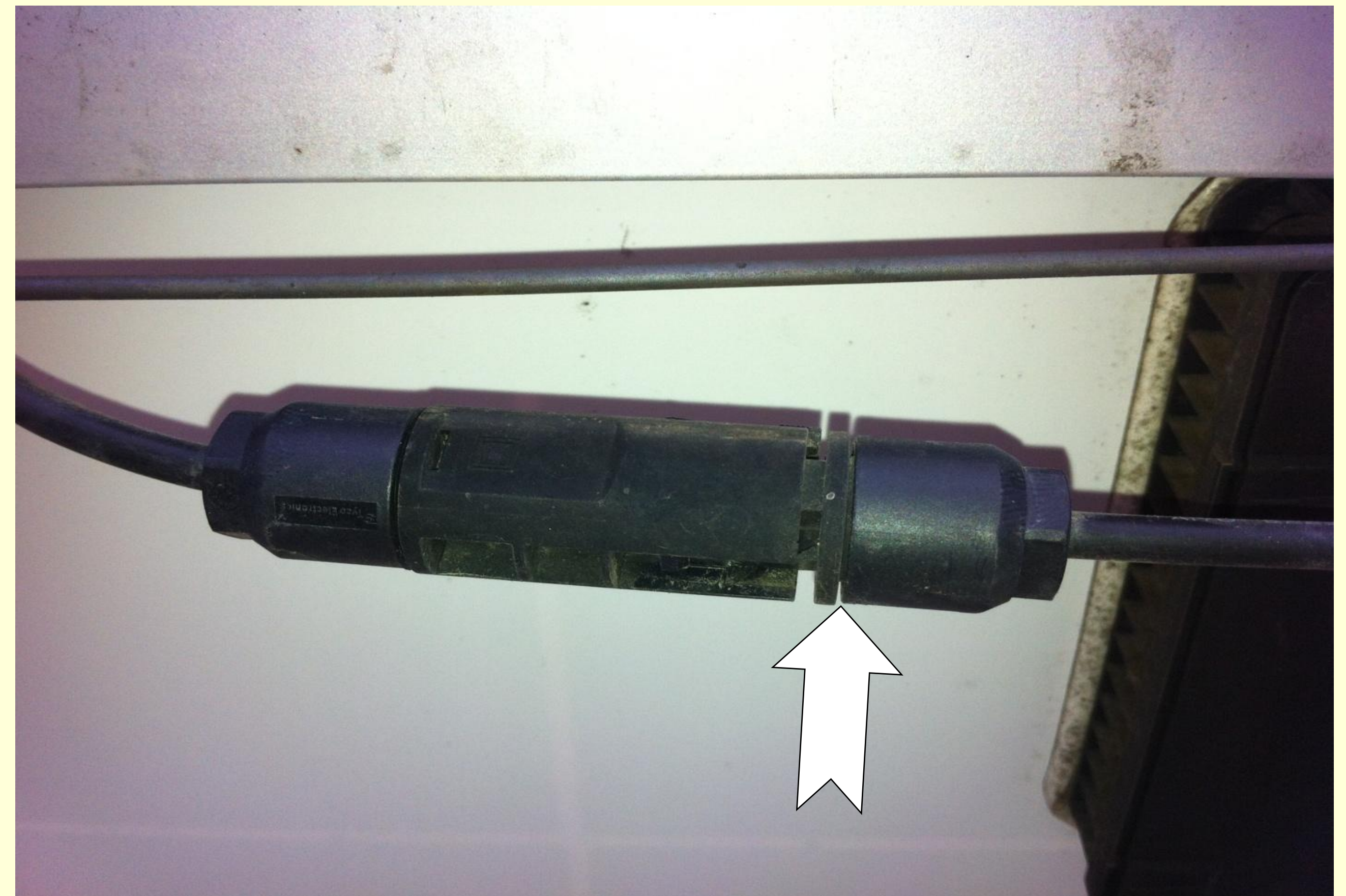
3. Gap of 2-3 mm opens up between mating connectors without any obvious external damage, external stress or fracture in latches
