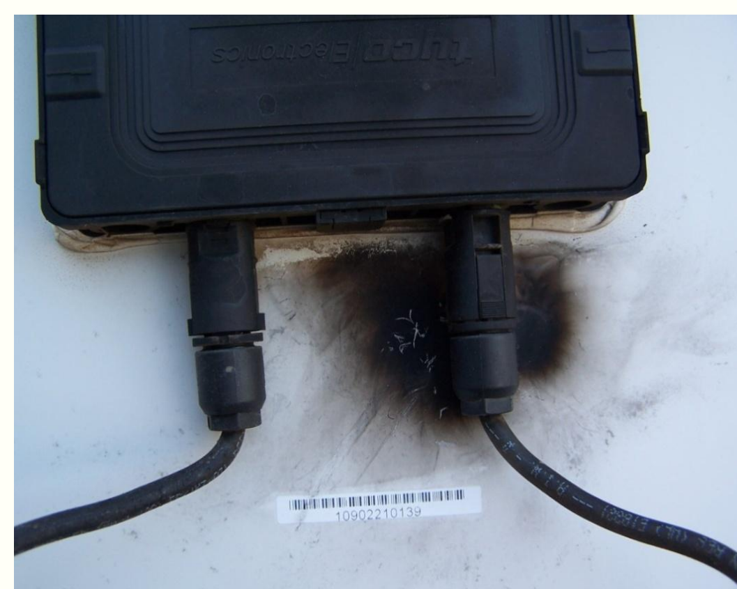
2. Connector failures at junction box
