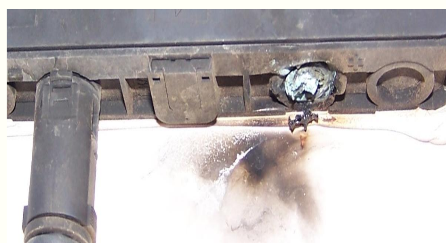
2. Connector failures at junction box
