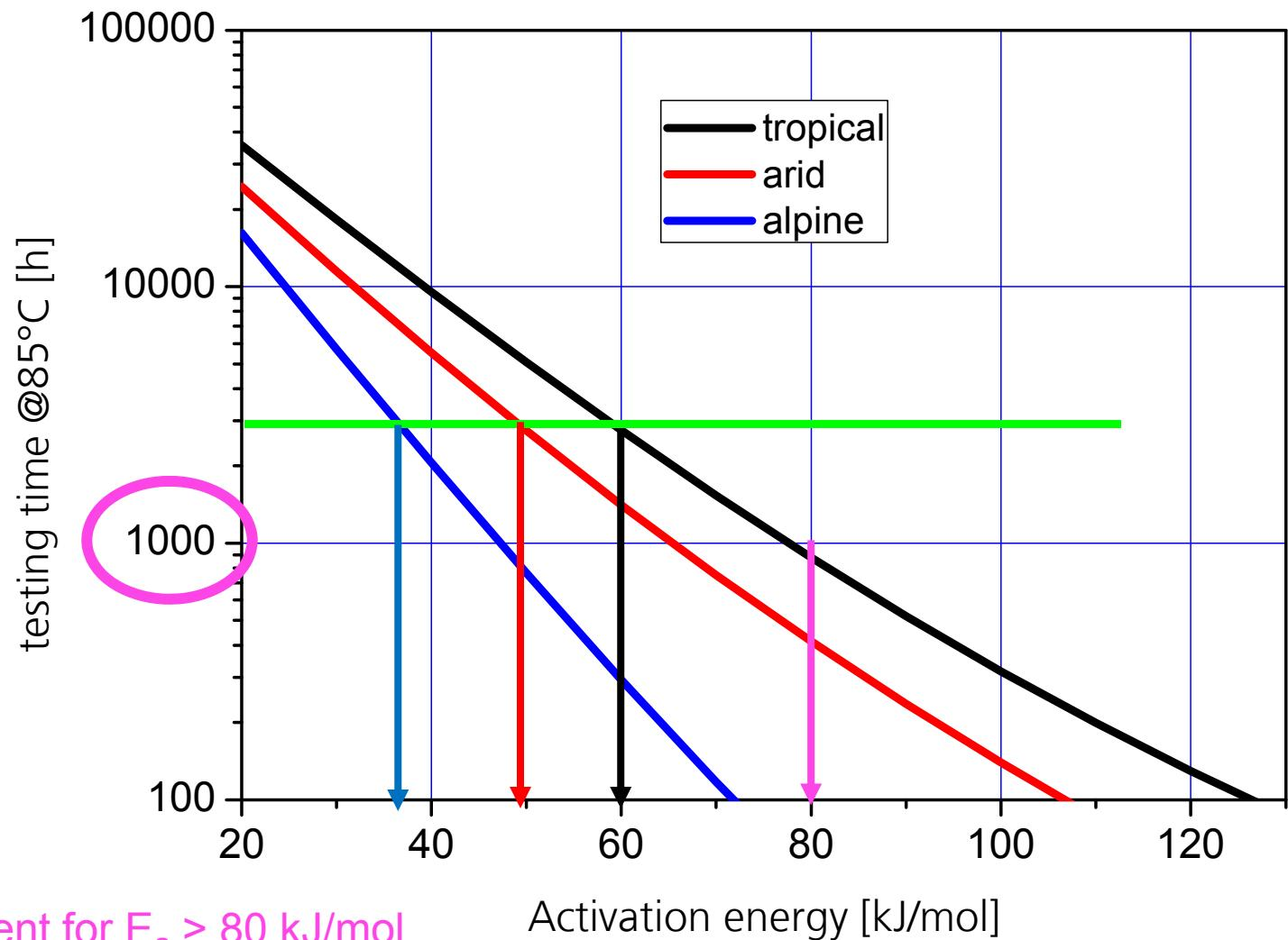
Type approval test would be sufficient for  $E_a > 80 \text{ kJ/mol}$
