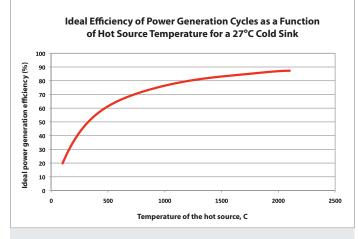
This chart illustrates the ideal efficiency of power generation cycles as a function of the temperature at which heat is transfered. The higher the temperature of heat transfer, the higher the cycle efficiency, and thus, the need for heat transfer fluids (HTFs) operating between 650° and 1200°C. *Graphic from Argonne*
