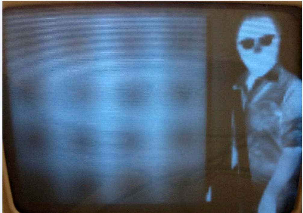
Thermal camera view of hot glass sheet cooled from behind by jet nozzles in a square grid
