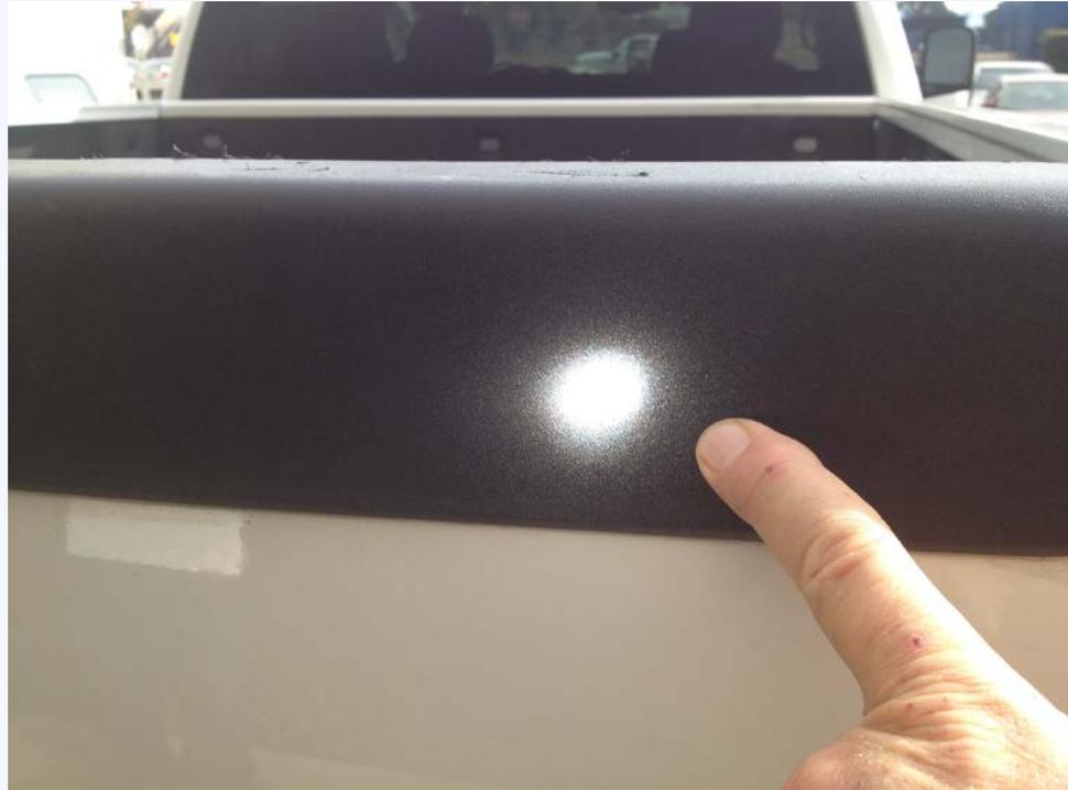
This pickup truck makes a handy screen to check solar image quality. A perfect solar image would be for the 1.7 m focal length would be 0.56” diameter.
