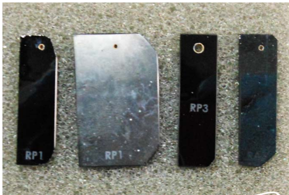
PDC Coupons for Molten Salt Testing
