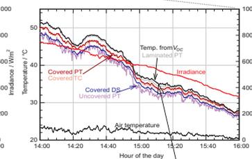
High temperature noise of uncovered PT due to air flow at the back side.
