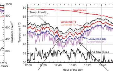
DS sensor exhibits lowest temperature despite insulation.
