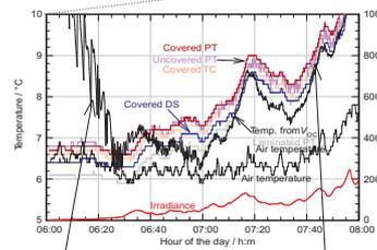
$V_{oc}$  method has low accuracy at low irradiances.
