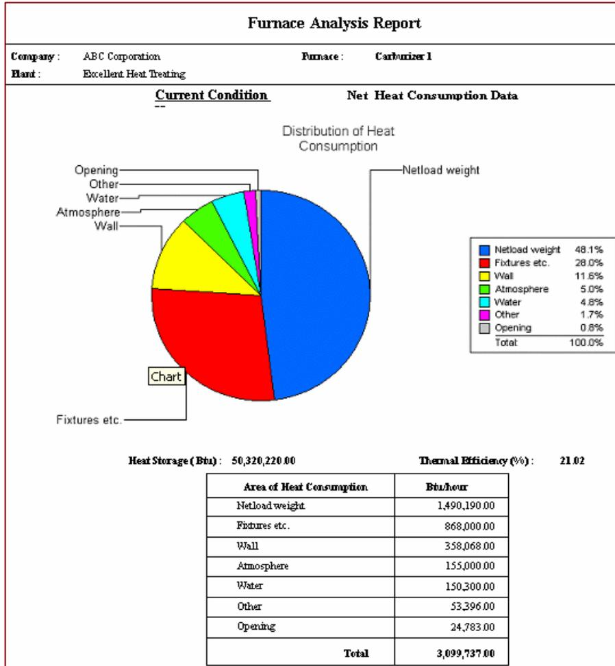
□ Analysis of energy used in part of a furnace under a given operating condition.
