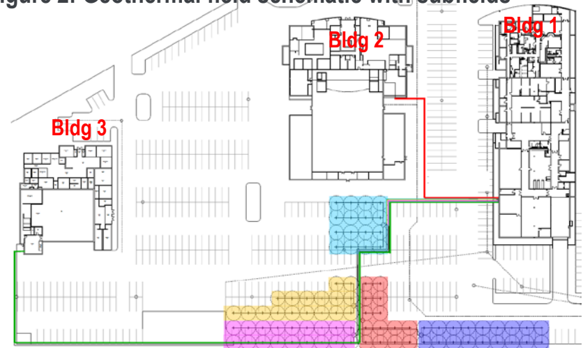
Figure 2: Geothermal field schematic with subfields
