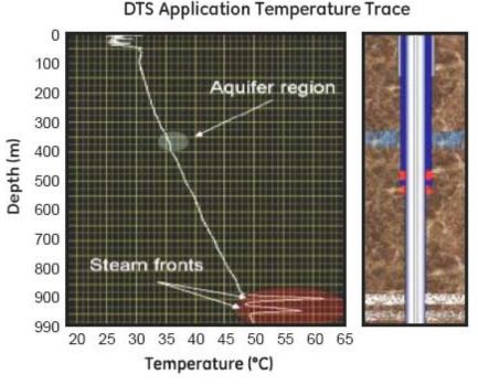
The effects of injection into the stimulation well are clearly seen when using DTS to monitor the recovery well to 1km deep
