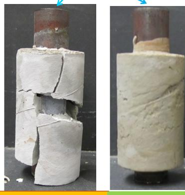
Class G/quartz flour New cement sheath cement sheath after 1 cvcle
