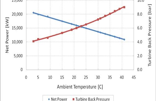
Study results for a 20-MW air cooled power plant simulation.
