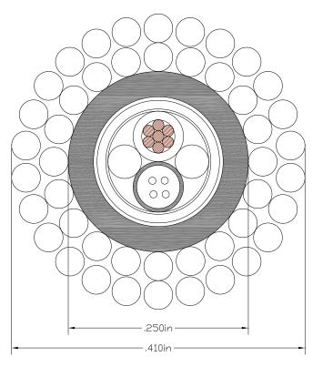
Complete Fiber/Copper Cable Solution for Long-Term Temperature and Pressure Measurement in Supercritical Reservoirs and EGS Wells
