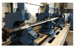
4¾-in. metal-metal motor flow loop test
