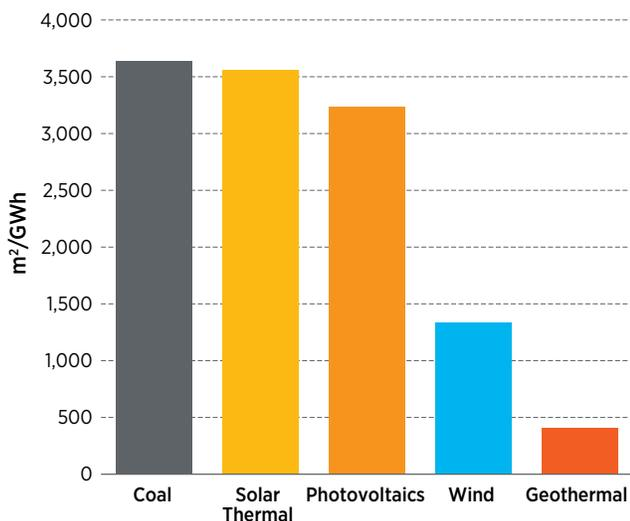
**Figure 2-16.** Land footprint by GWh<sub>e</sub> for various electricity-generation technologies
