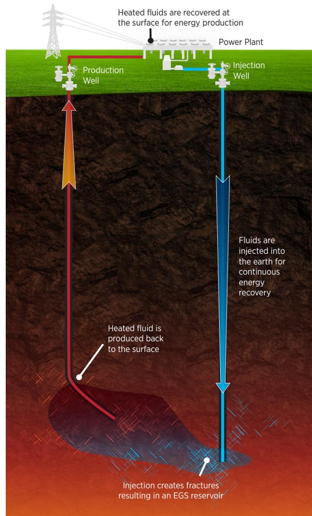
**Figure 2-6.** Conceptualization of an enhanced geothermal system
