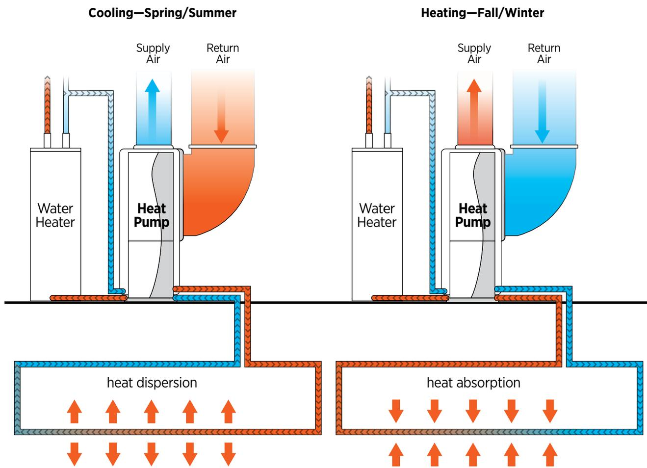
**Figure 2-12.** Schematic of a geothermal heat pump showing the simplified ground heat-exchanger loop, heat pump, and indoor delivery system
