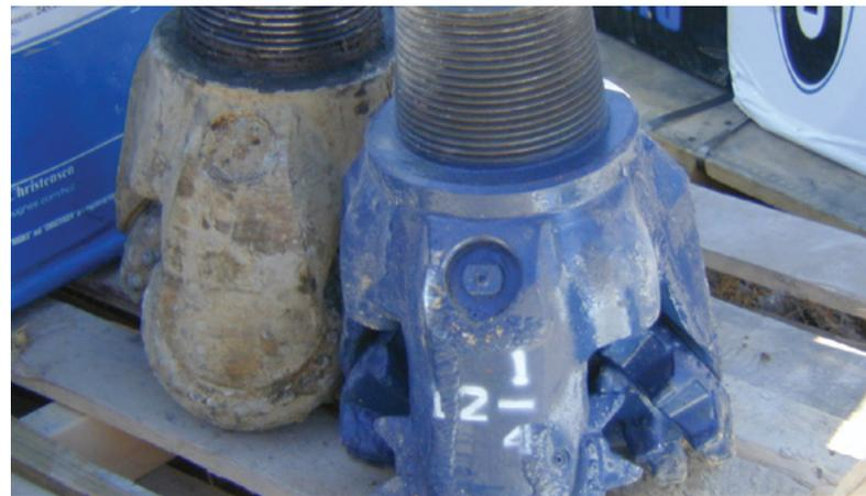
Drill bits used at the Raft River geothermal site in Idaho.
