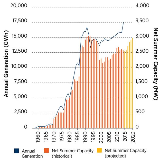
**Figure 2-9.** U.S. historical annual geothermal electricity generation (in GWh<sub>e</sub>) and installed net summer capacity (in MW<sub>e</sub>)
