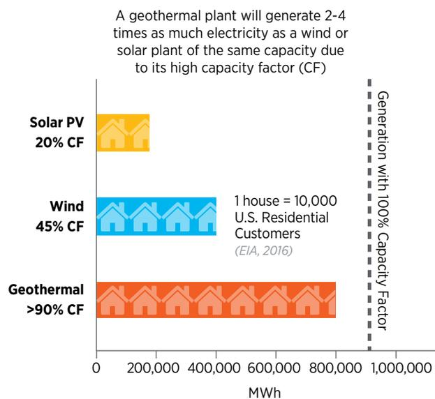
**Figure 2-14.** Capacity factors for geothermal, wind, and solar photovoltaic indicating annual generation (MWh<sub>e</sub>) from equivalent 100-MW<sub>e</sub> nameplate-capacity power plants
