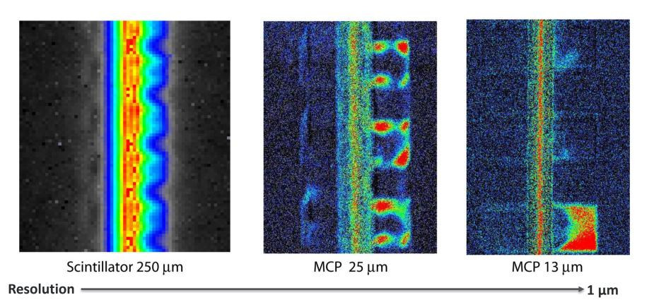
Easily resolve water content in gas diffusion layer at 25 μm resolution
