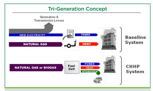
Tri-generation, or combined heat, hydrogen, and power (CHHP), systems can locally produce useful power, heat, and fuel with low emissions and high efficiency that avoids the energy and emissions penalties of transmission/transportation of traditional methods.
