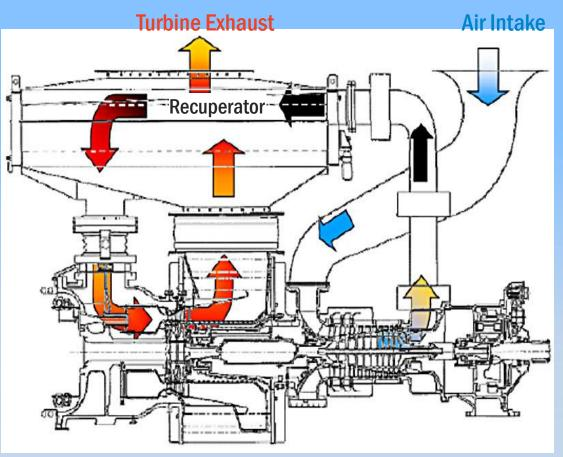
Combustor | Turbine | Compressor | Gearbox
