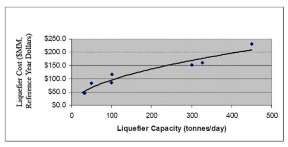
Figure 6.1.2. Liquefier cost versus design capacity (National Renewable Energy Laboratory, 2006)
