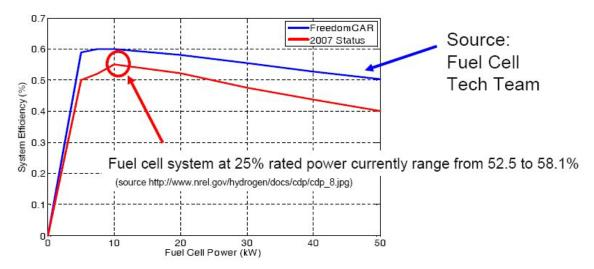
Figure 7.1.1. Fuel cell power versus system efficiency (Rousseau and Wallner, 2008)
