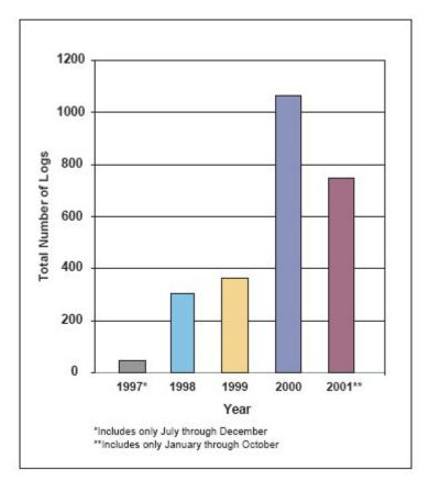
Figure 4.2.1. Transmission loading relief calls for 1997-2001 (Abraham, 2002)
