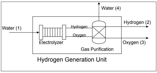
Figure 5.2.2. Distributed electrolysis mass balance diagram (Ramsden, 2008b)
