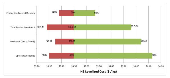
Figure 9.1.9. Production sensitivities for distributed natural gas pathway
