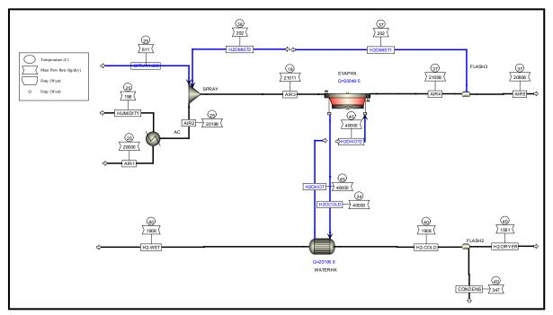
Figure 5.2.3. Distributed electrolysis process flow diagram cooling water detail (Ramsden, 2008b)
