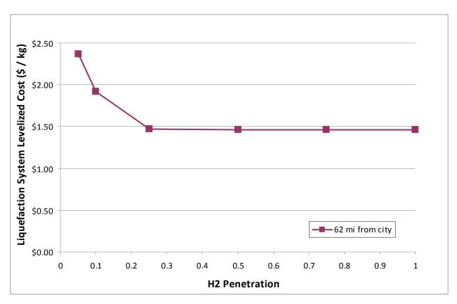
Figure 9.3.14. Liquefaction system levelized cost versus penetration for the central biomass–liquid truck delivery pathway
