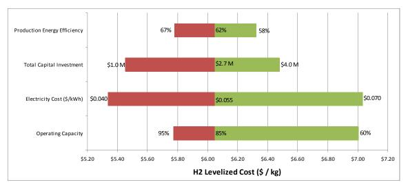
Figure 9.2.9. Production sensitivities for distributed electrolysis pathway
