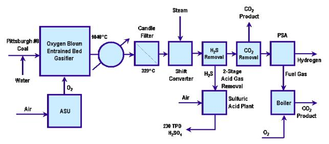
Figure 5.6.1. Central coal with carbon capture process flow diagram (Rutkowski, 2008a)
