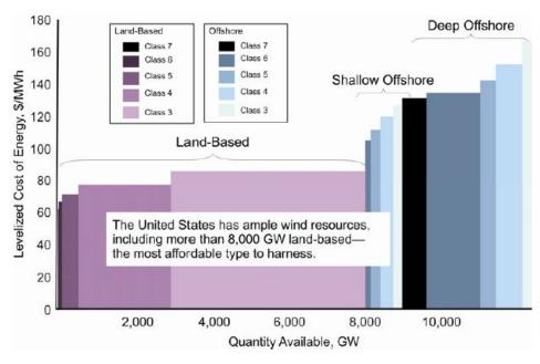
Figure 3.2.4. Wind energy supply curve (U.S. Department of Energy, 2008)
