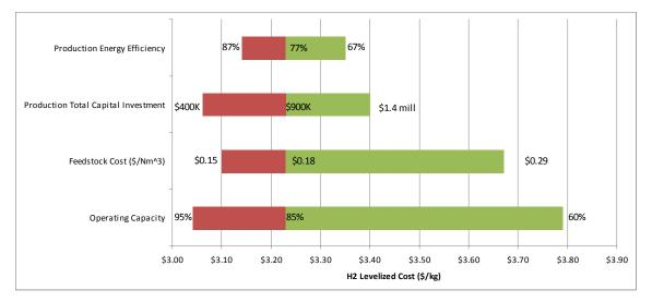
Figure 9.1.10. Production sensitivities for distributed natural gas pathway with advanced technology
