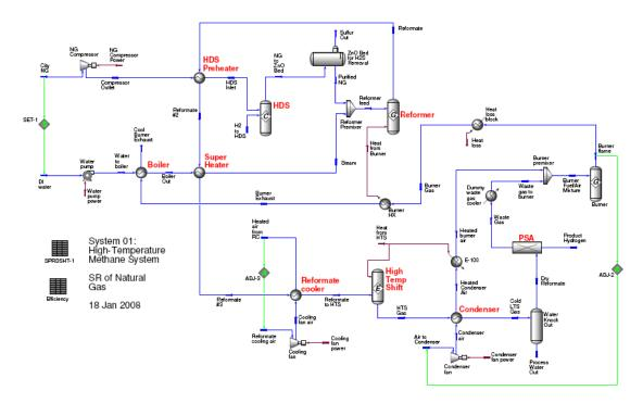
Figure 5.1.1. Distributed natural gas reforming process flow diagram (James, 2008)
