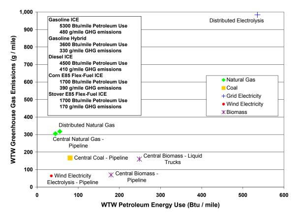
Figure 1.0.1. Comparison of pathways' petroleum use and greenhouse gas emissions
