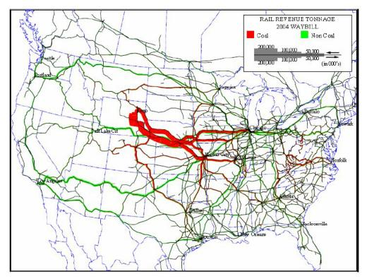
Figure 4.4.2. Rail traffic on the rail network for 2004 waybill sample data (McCollum, Ogden, and Chernicoff, 2007)
