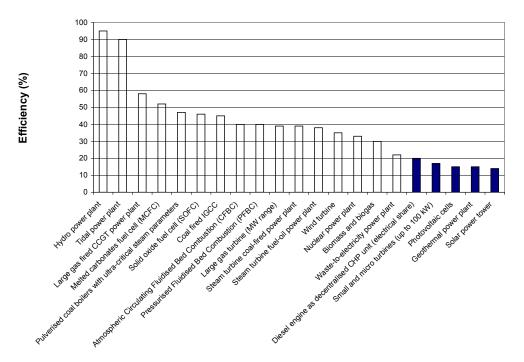
Figure 3.2.1. Efficiency in electricity generation from various sources (van Aart, 2004)
