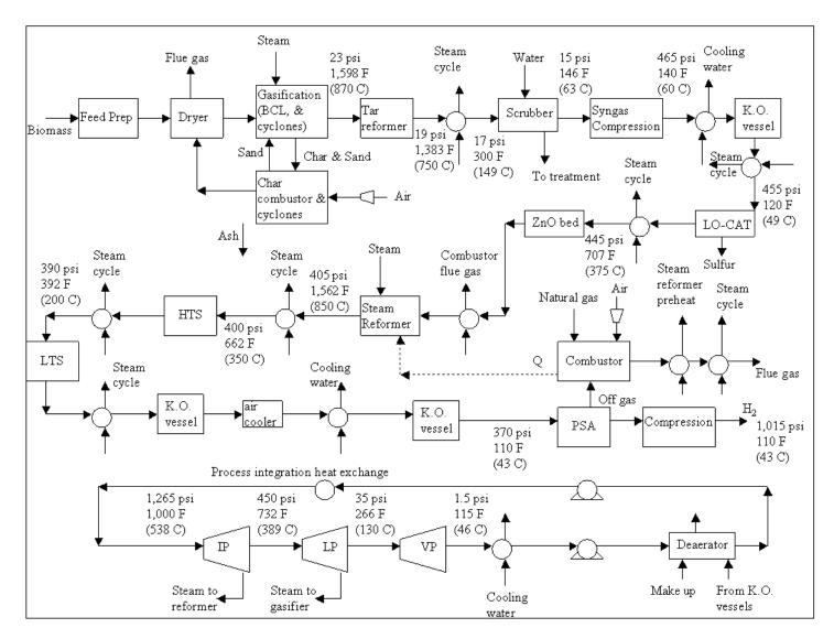
Figure 5.3.1. Central biomass gasification flow diagram (Mann and Steward, 2008)
