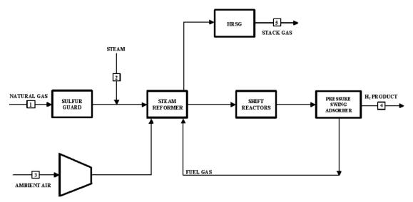
Figure 5.4.1. Central natural gas process flow diagram (Steward, 2008)
