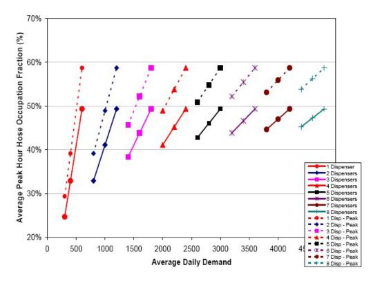
Figure 6.3.3. Recommended number of refueling station dispensers (Nexant 2008)
