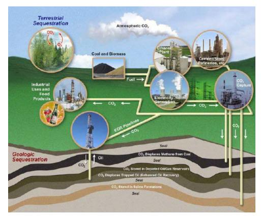
Figure 3.5.1. Geological and terrestrial sequestration (National Energy Technology Laboratory, 2008)
