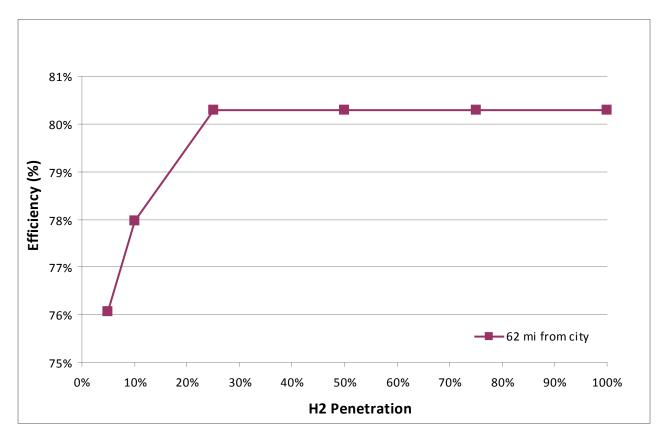
Figure 9.3.16. Liquefaction system efficiency versus penetration for the central biomass– liquid truck delivery pathway
