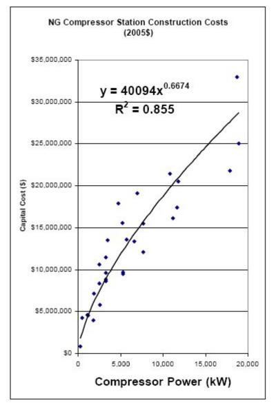
Figure 6.2.1. Compressor cost as a function of power draw (National Renewable Energy Laboratory, 2006)
