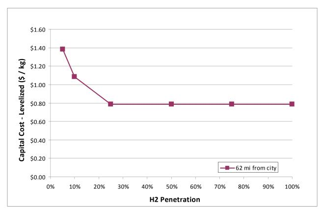
Figure 9.3.15. Liquefaction system capital cost (levelized) versus penetration for the central biomass–liquid truck delivery pathway
