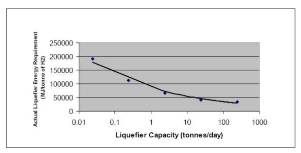
Figure 6.1.1. Liquefier energy requirement versus hydrogen flow rate (National Renewable Energy Laboratory, 2006)
