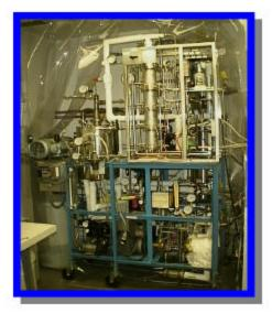
Figure 7. Epyx fuel processor and LANL PROX.
