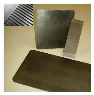
Figure 1. Compression- and injection-molded bipolar plates.
