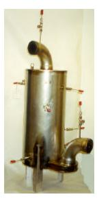
Figure 2. Low-temperature shift converter test article.
