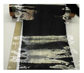
Figure 3. 3-layer catalyst-coated membrane as a rollgood.
