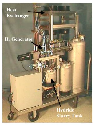
Figure 2. 50-kWe hydrogen generation system.
