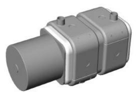
Figure 8. Motor/compressor/expander integrated for testing.
