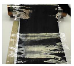
3M's Three-Layer Catalyst-Coated Membrane
