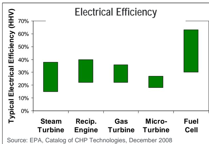
Fuel cells convert chemical energy directly into electrical energy, bypassing inefficiencies associated with thermal energy conversion
