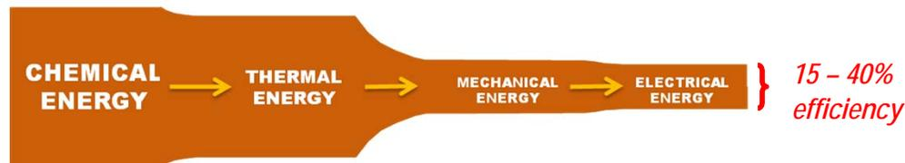
**Fuel cells** — convert chemical energy directly into electrical energy, bypassing inefficiencies associated with thermal energy conversion. Available energy is equal to the Gibbs free energy.
