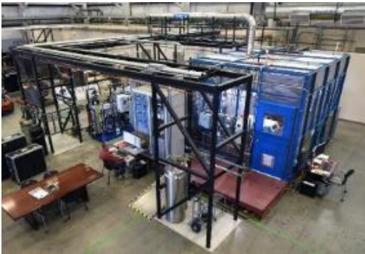
25 kW high-temperature electrolysis @ INL Energy Systems Laboratory
