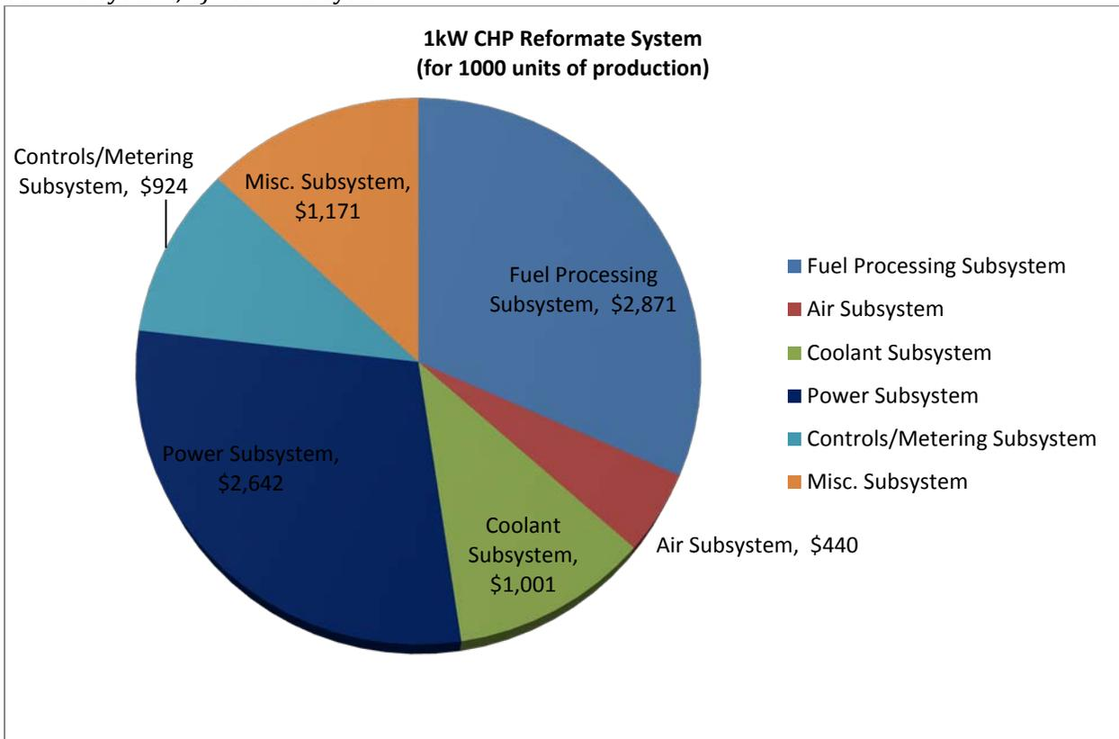
a) Subsystem cost breakdown of CHP system with reformat fuel (1 kWe system)
