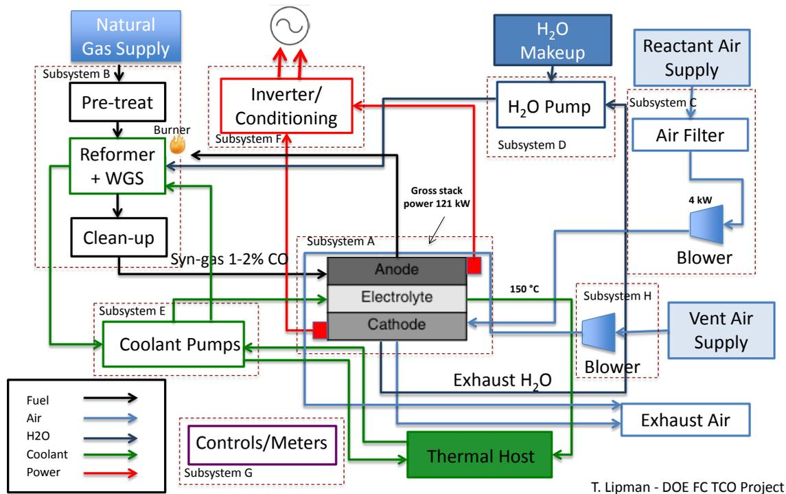
Figure 1.1. CHP with reformate fuel system schematic for 100kWe HT PEM FC system.
