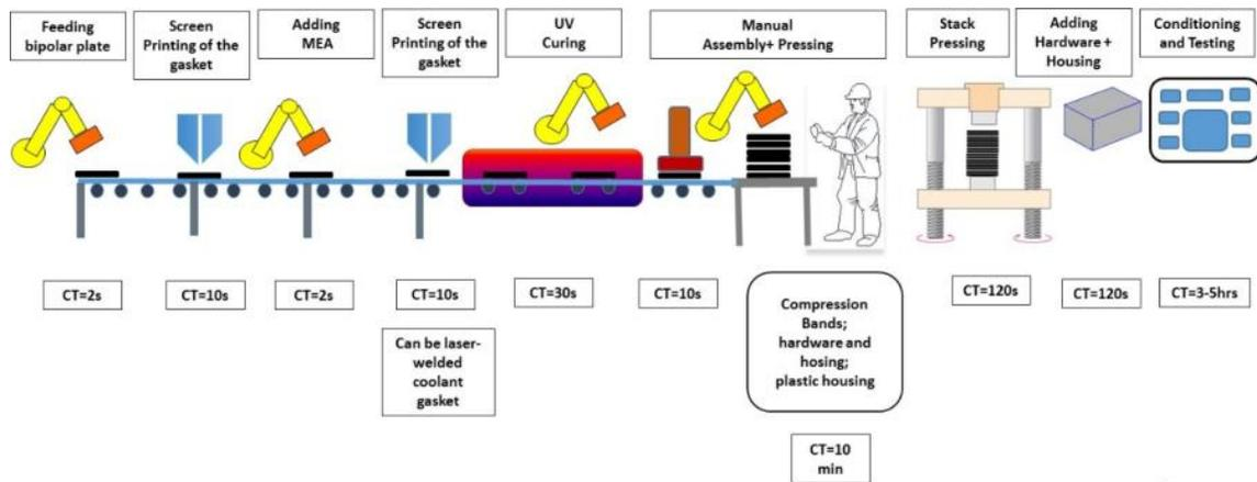
Figure 2.25. Process flow for semi-automatic assembly line
