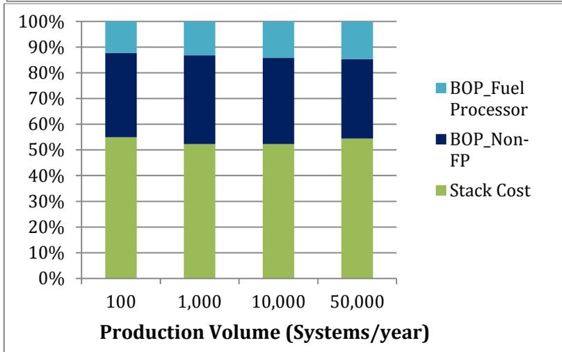
Figure C. 4: Subsystem percentage cost breakdown for CHP system with reformate fuel
