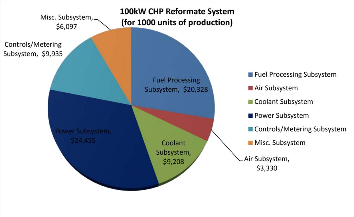
d) Subsystem cost breakdown of CHP system with reformat fuel (100 kWe system)
