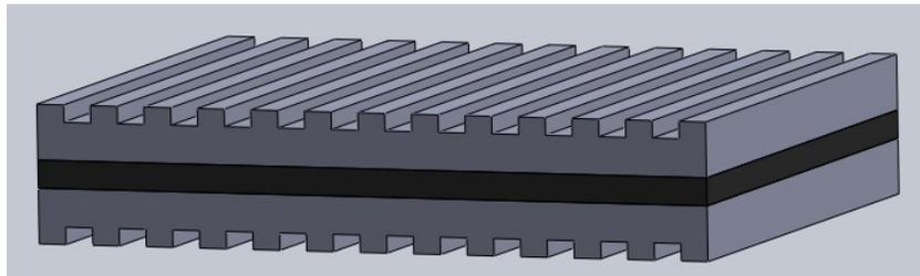
Figure 2.15. Half Plate with Separator Layer
