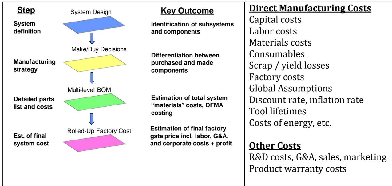
Figure A.1 (a) Generalized roll-up steps for total system cost; (b) scope of direct manufacturing costs for components produced in-house.
