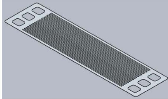
Figure 2.14. Bipolar Half Plate for Low Temperature PEM Fuel Cells
