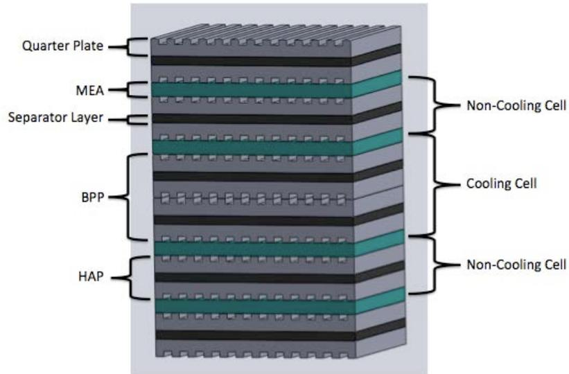
Figure 2.17. HT PEM fuel cell stack configuration
