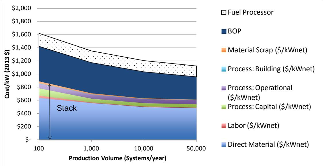
Figure C.3. HT PEM fuel cell system cost breakdown for CHP system with reformate fuel.
