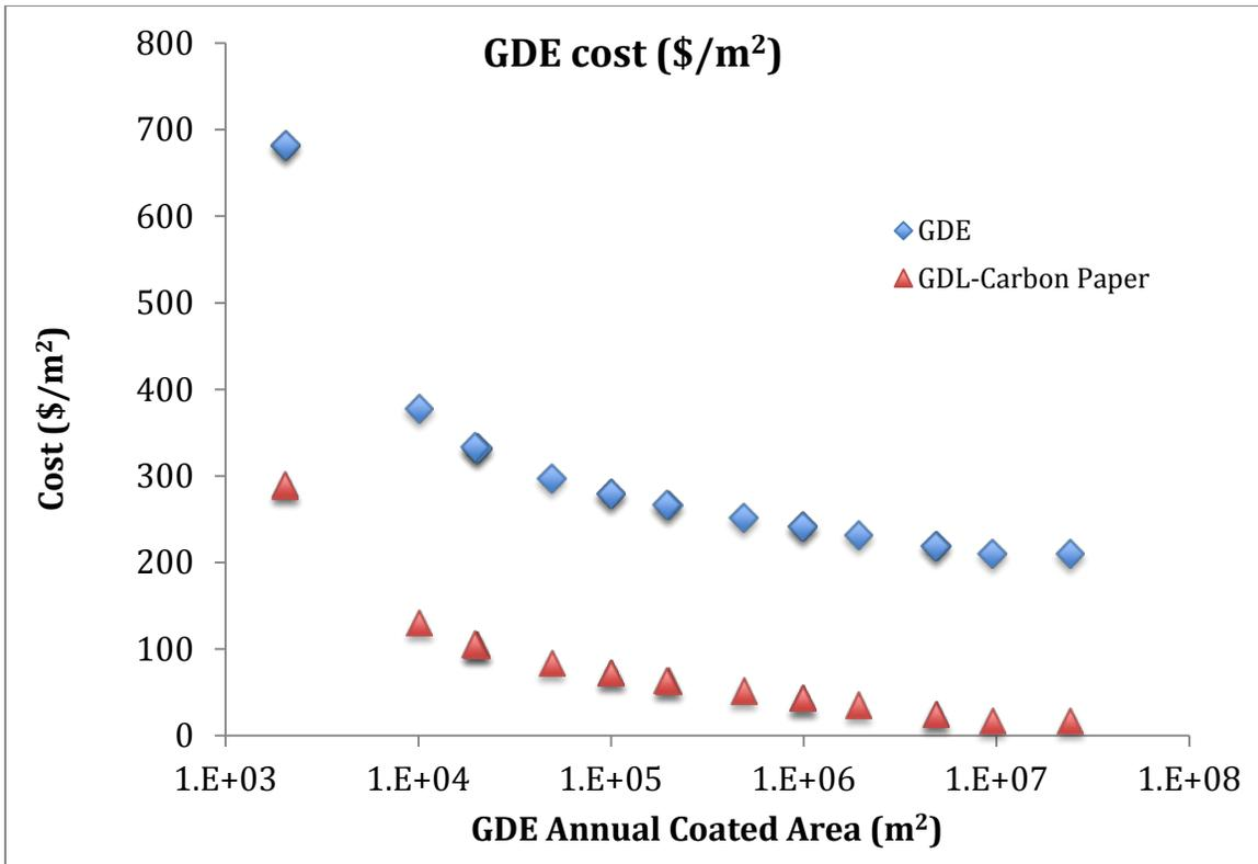
Figure 2.9. Gas diffusion electrode (GDE) cost along with carbon paper cost in (\$/m<sup>2</sup>) with annual production volumes
