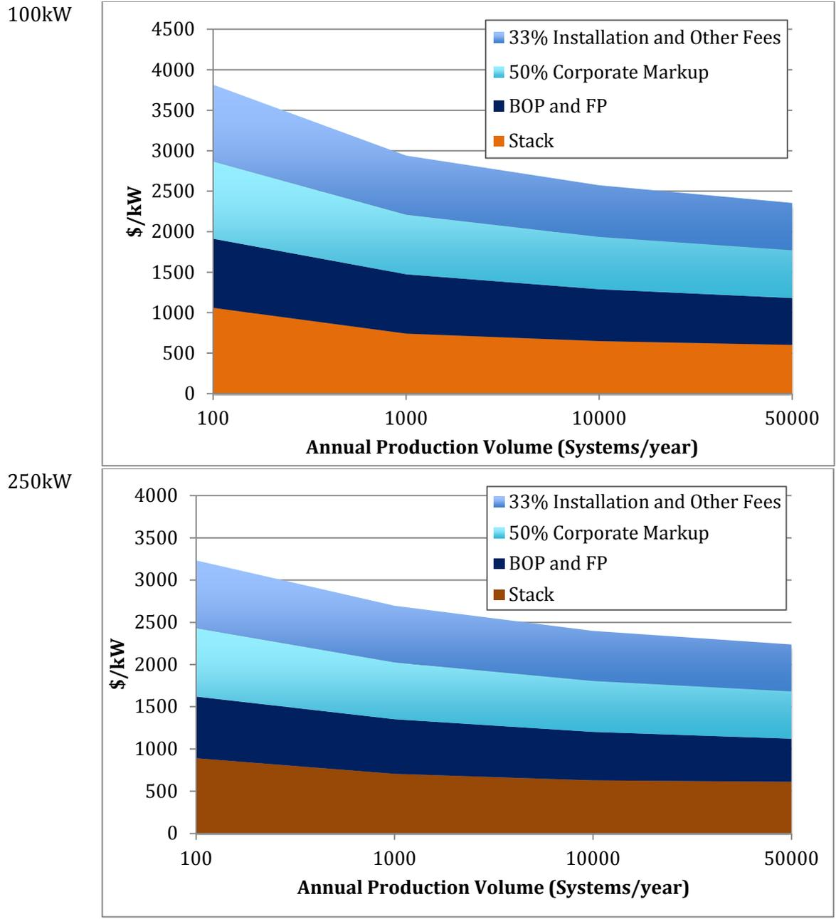
Figure C.6: Installed costs of the CHP HT PEMFC system
