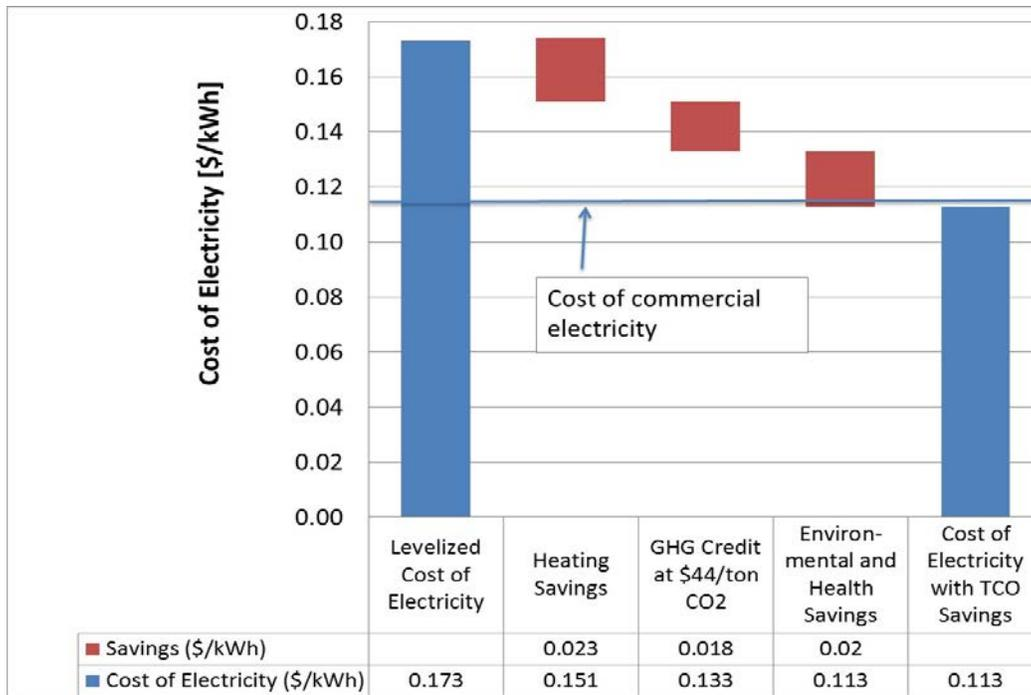
Figure D.1. Levelized and total cost of electricity for a 50kW small hotel in Chicago, IL.
