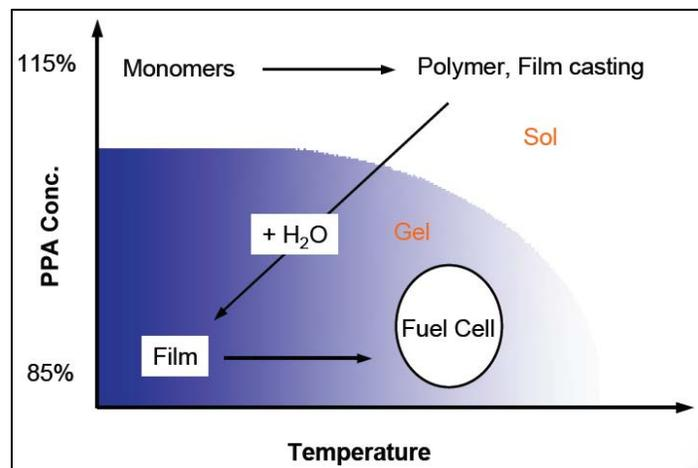
Figure 2.2. Hydrolysis and doping are made to get more stable membrane (Hydrolysis @ $T=25^{\circ}\text{C}$ ;  $\text{RH}=40\pm 5\%$ ) (Seel et al., 2009)
