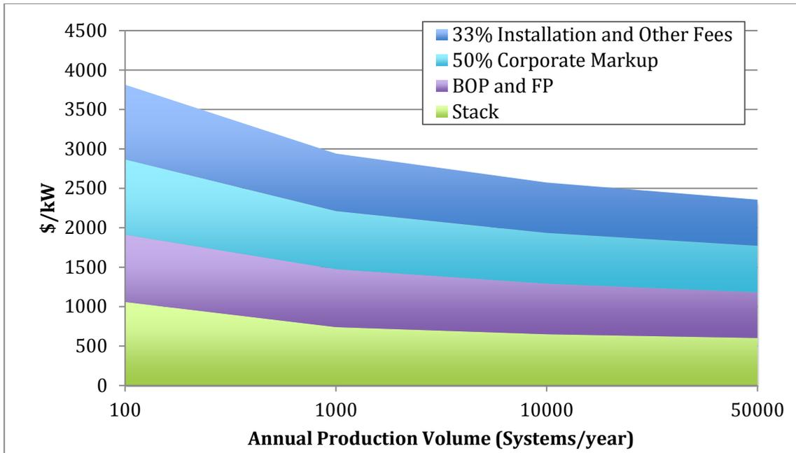
Figure 4.4. Installed cost as a function of volume for 100kW CHP system.
