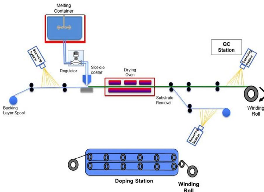
Figure 2.3. Schematic of the casting process and in situ quality control of PBI-based membrane
