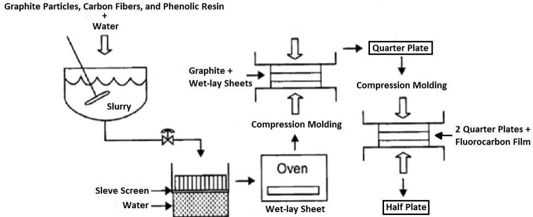
Figure 2.19. Wet-Lay Compression Mold Diagram (Baird, 2004)
