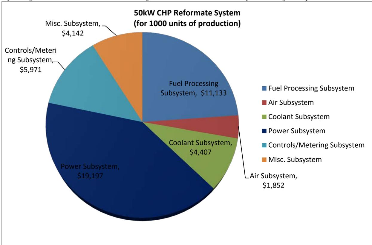
c) Subsystem cost breakdown of CHP system with reformat fuel (50 kWe system)
