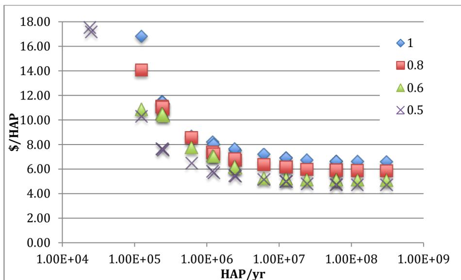
Figure 2.23. Sensitivity analysis for compression molding pressure requirement (the legend refers to the multiplication factor of the nominal plate molding pressure)
