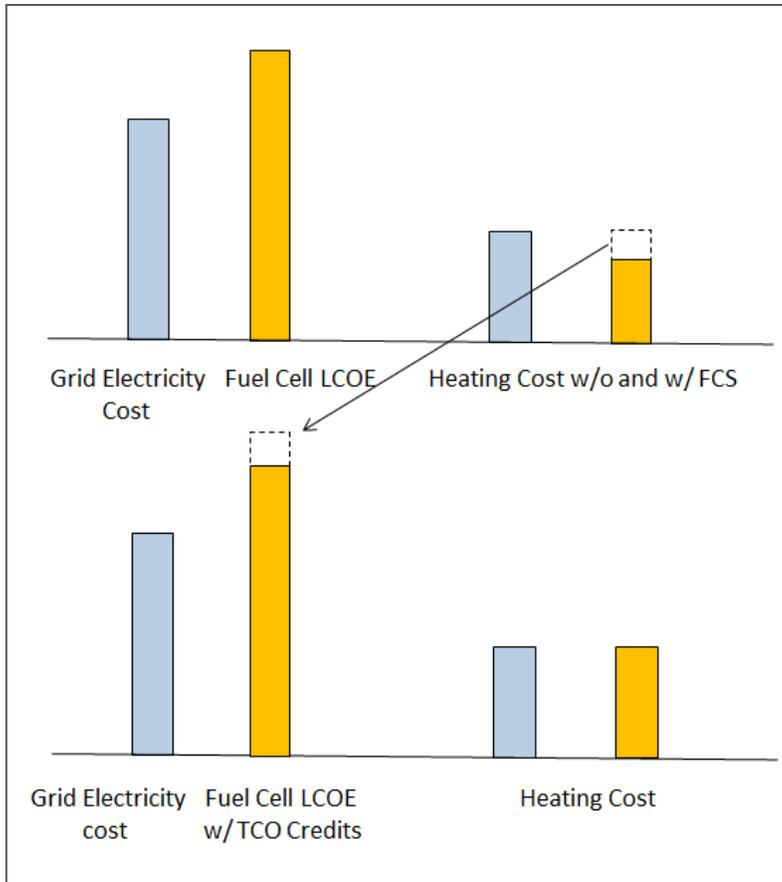
Figure 5.2. Cost of energy service for FC CHP and conventional electricity and heating systems. A fuel cell CHP system will typically increase the levelized cost of electricity (upper left two bars). But if waste heat is utilized, the cost of heating is reduced (upper right two bars). In this treatment, all non-electricity credits (heating, carbon, etc) are applied to a “total cost of electricity” (lower left two bars).
