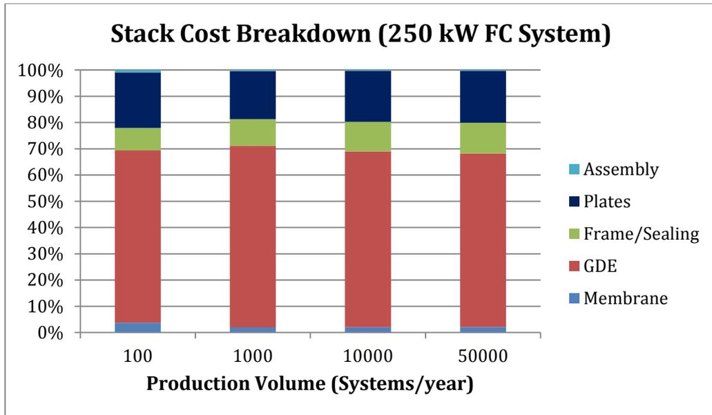
Figure C. 5: Stack cost percentage cost breakdown for CHP system with reformat fuel
