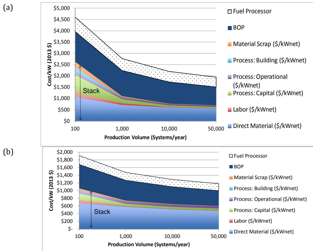
Figure 4.1. System cost vs annual production volume for (a) 10kWe and (b) 100kWe HT PEM CHP system with reformat fuel.
