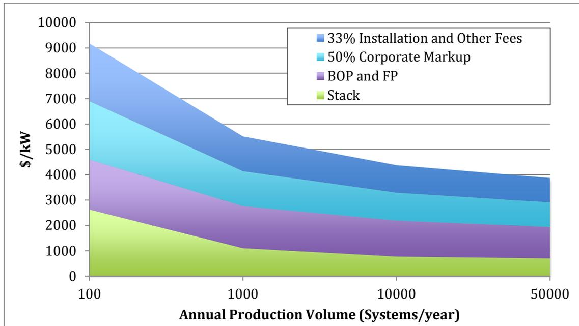
Figure 4.3. Installed cost as a function of volume for 10kWe CHP system.
