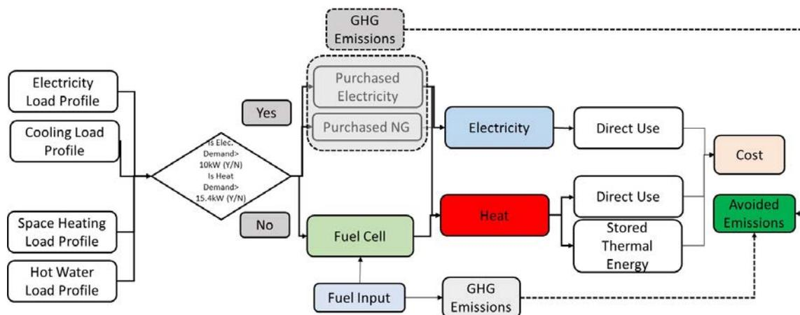
Figure 5.1. Flow chart and logic used to model 10kWe CHP system with reformat fuel.
