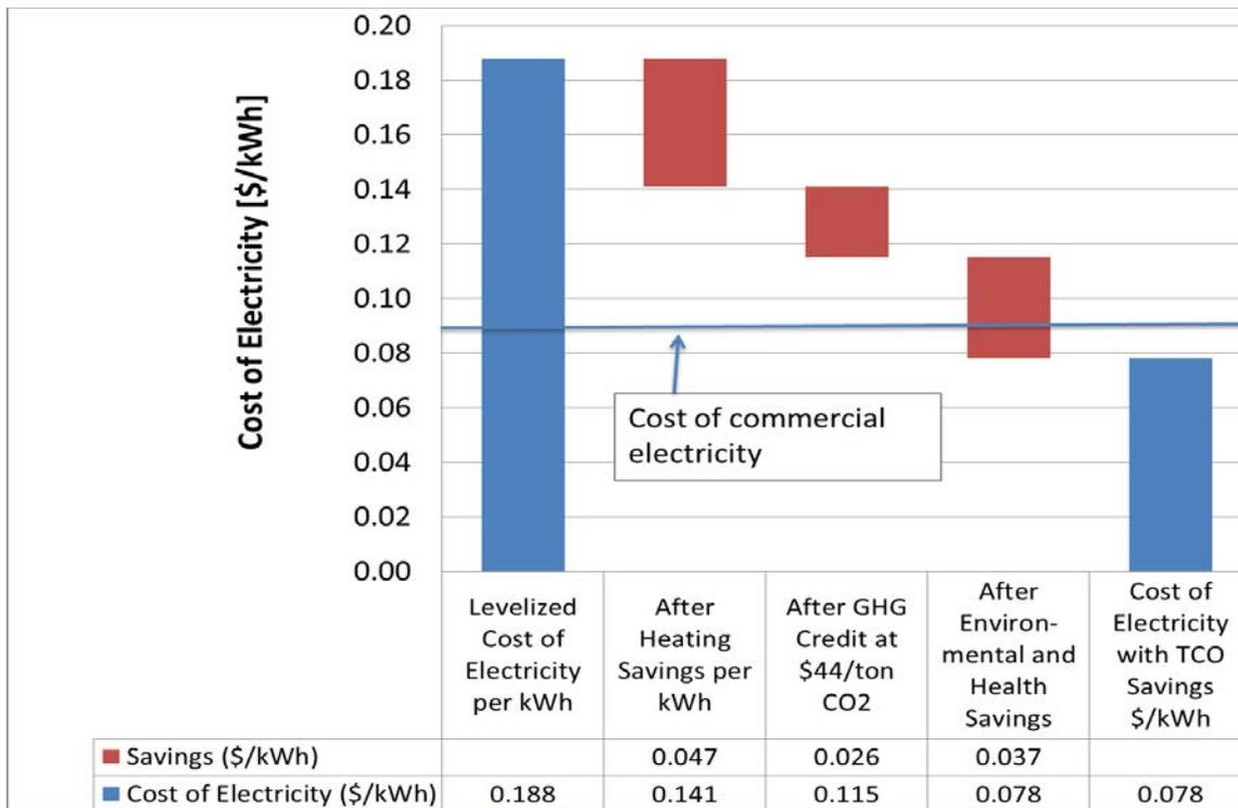
Figure 5.3. Levelized and total cost of electricity with TCO credits for a 10kWe small hotel in Chicago, IL for a FC system assumed to provide space heating and water heating.
