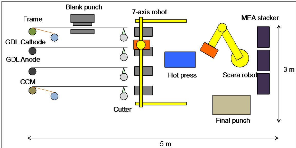
Figure 2.11. MEA Frame process flow
