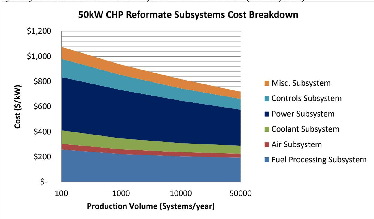
b) Subsystem cost breakdown of CHP system with reformate fuel (50 kWe system)
