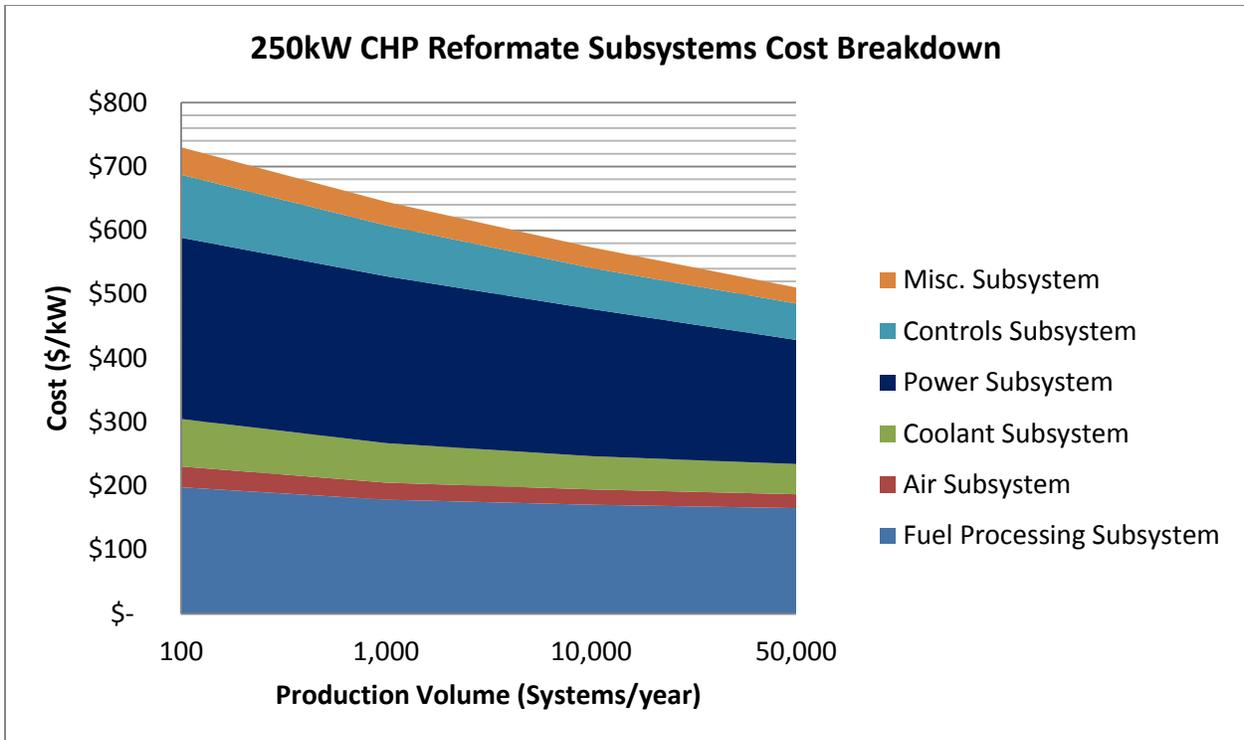
c) Subsystem cost breakdown of CHP system with reformate fuel (250 kWe system)
