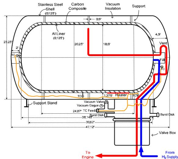
Fig. 1. Design schematic of the LLNL cryo-tank.
