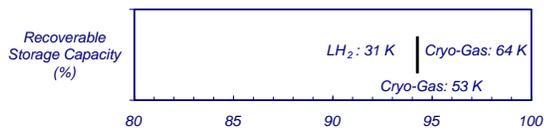
Recoverable storage capacity depends on minimum delivery pressure and heat input
