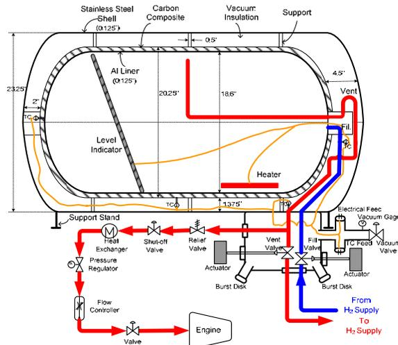
Fig. 4. Modified cryo-tank.
