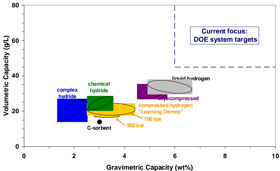
Figure 1 shows the capacity of cryo-compressed tanks reported in Table 1 compared to the current state of the art for other hydrogen storage options. Note that the values in Figure 1 represent a snapshot in time and are periodically assessed and updated by DOE (see: [http://www1.eere.energy.gov/hydrogenandfuelcells/storage/tech\\_status.html](http://www1.eere.energy.gov/hydrogenandfuelcells/storage/tech_status.html)).
