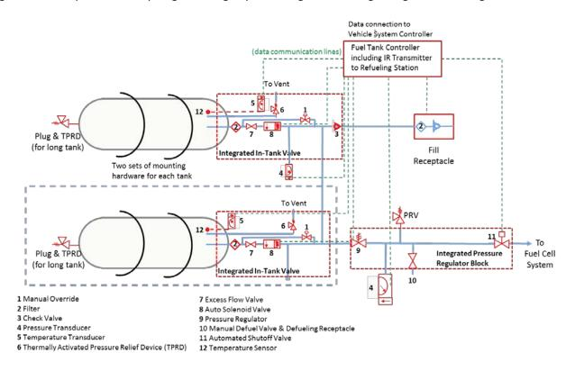
Figure 1b: Example 700 bar Hydrogen Storage System Diagram Showing a Dual-Tank Configuration
