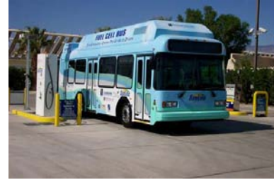
Figure B-4. ThunderPower fuel cell bus
