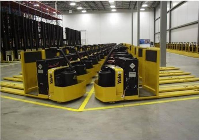
Central Grocers has purchased 221 Yale forklifts powered by PlugPower GenDrive PEM fuel cells for their distribution center in Joliet, Illinois. Air Products is providing the hydrogen gas and fueling stations.
