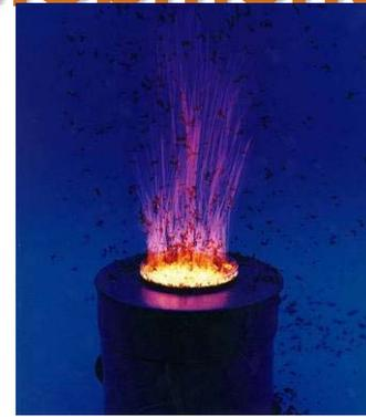
Glycine – nitrate powder synthesis of  $\text{La}_{0.7}\text{Ca}_{0.31}\text{CrO}_3$
