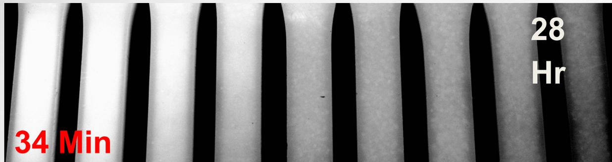
Graphic showing the progression of blistering formation in McMaster LDPE with time after removal from high pressure H<sub>2</sub>.
