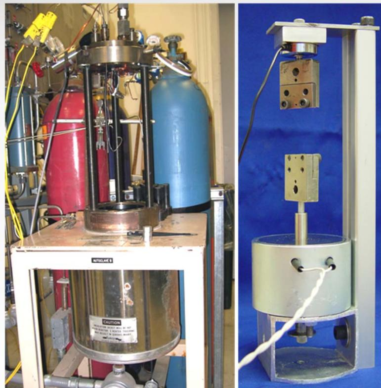
Figure 1: (RIGHT) The high pressure hydrogen autoclave can accommodate up to 5" diameter x 10" height. (LEFT) A photograph of the partially completed in-situ tensile rig. LVDT is not shown.
