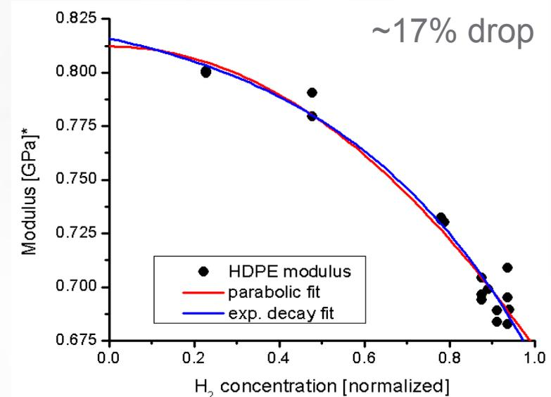
HDPE modulus is negatively impacted as a function of H<sub>2</sub> absorption, but recoverable.
