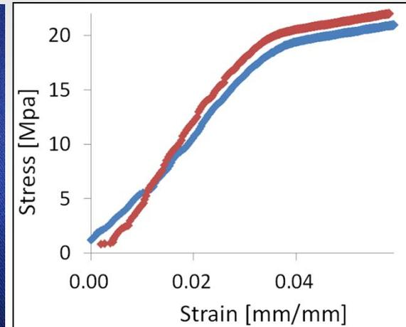
Left: HDPE tensile samples before and after testing in 4,000 psi hydrogen. Right: Preliminary data from in-situ tensile rig. (Red) data is for HDPE pulled in air, and (blue) data is for an identical HDPE sample pulled in 4,000 psi hydrogen. Hydrogen data shows a lower modulus defined by the initial slope
