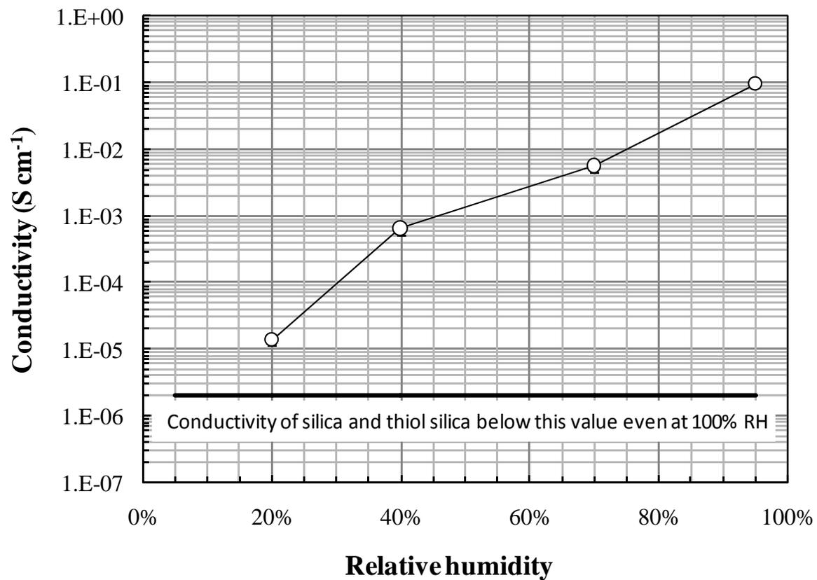
**Sulfonic Acid functionalized silica shows respectable pellet conductivities**
