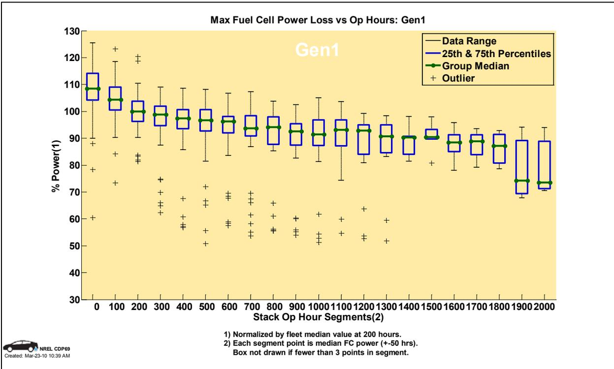
Figure 39: Maximum fuel cell power degradation—Gen 1 (CDP69)
