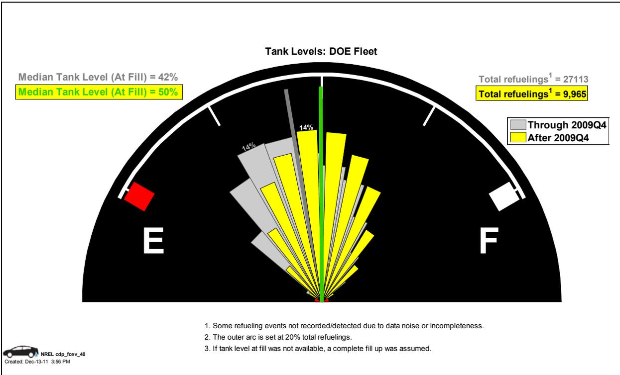
**Figure 117: Hydrogen tank level at fueling (CDP40)**
