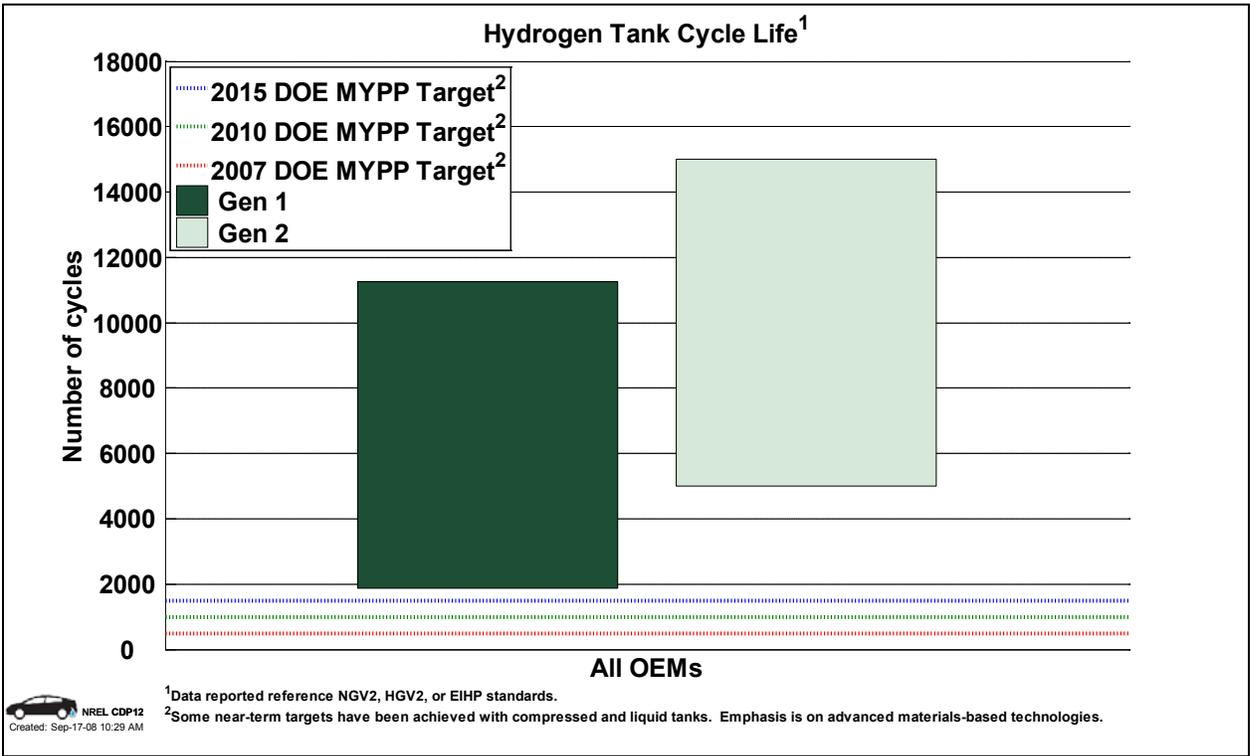
Figure 33: Vehicle hydrogen tank cycle life (CDP12)
