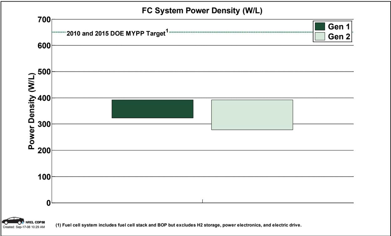
**Figure 35: Fuel cell system power density (CDP58)**
