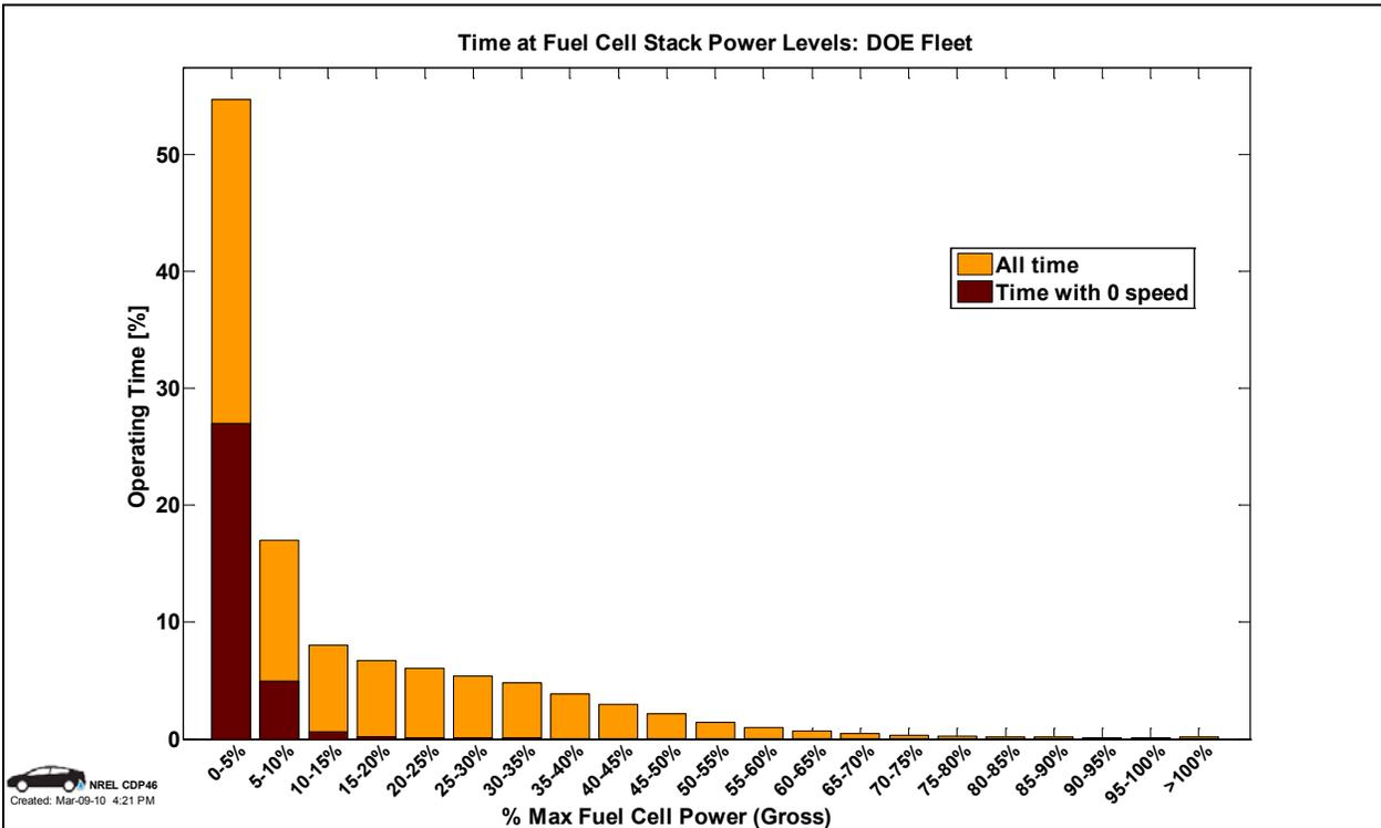
Figure 14: Fuel cell system operating power (CDP46)
