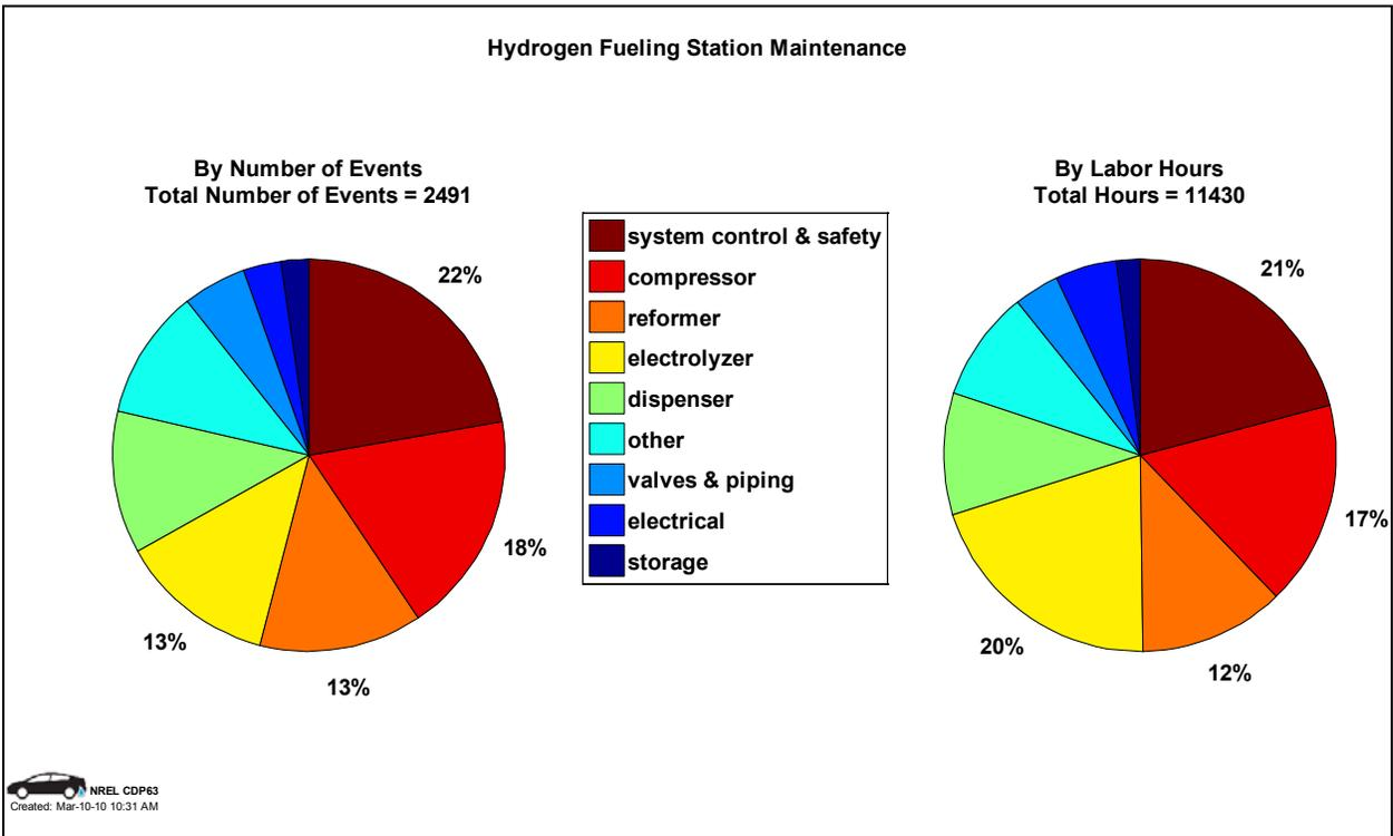
Figure 100: Hydrogen fueling station maintenance by system (CDP63)
