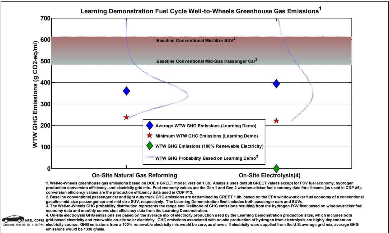
Figure 76: Learning Demonstration vehicle greenhouse gas emissions (CDP62)
