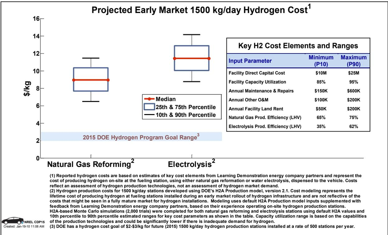
Figure 78: Hydrogen production cost vs. process (CDP15)
