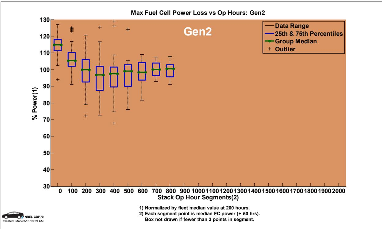
Figure 40: Maximum fuel cell power degradation—Gen 2 (CDP70)
