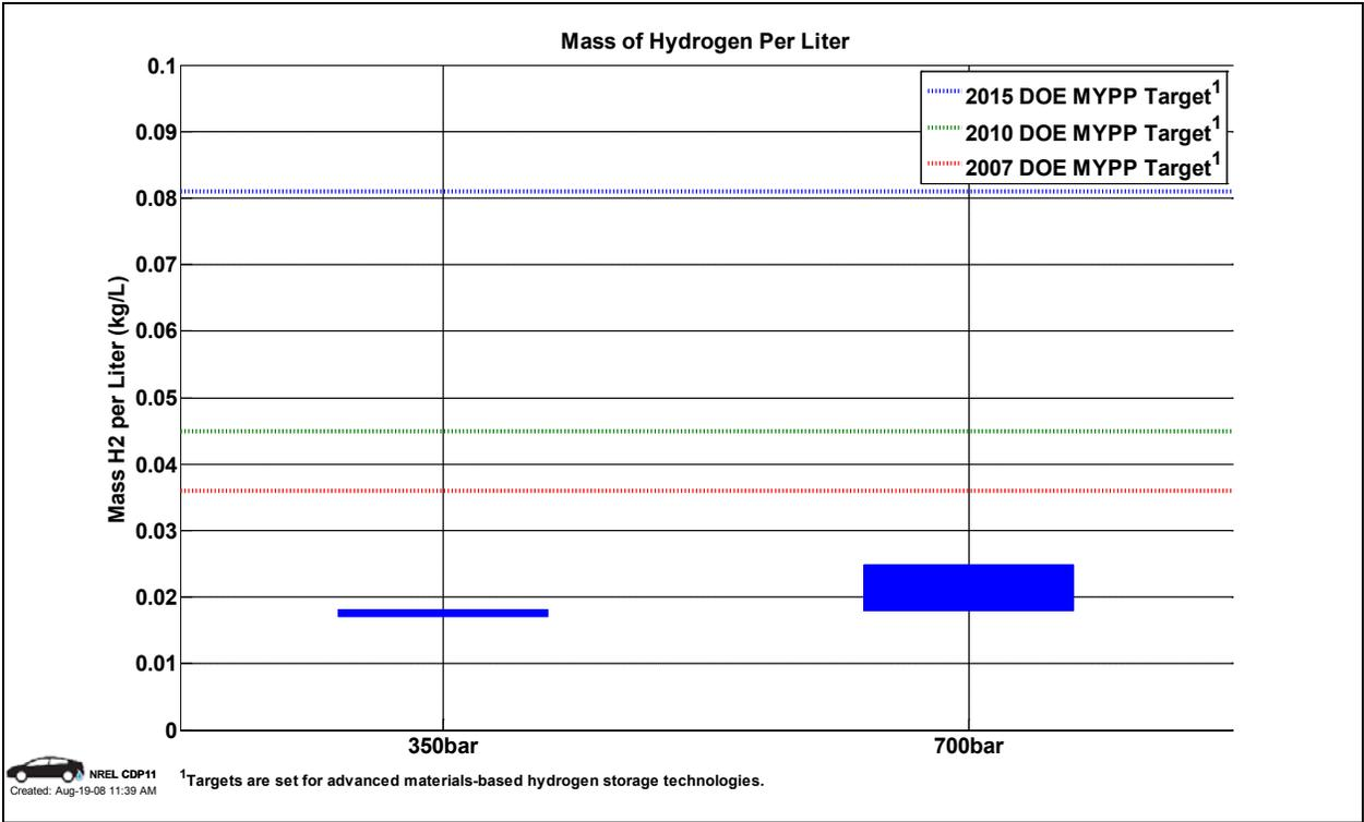
**Figure 31: Volumetric capacity of hydrogen storage (CDP11)**
