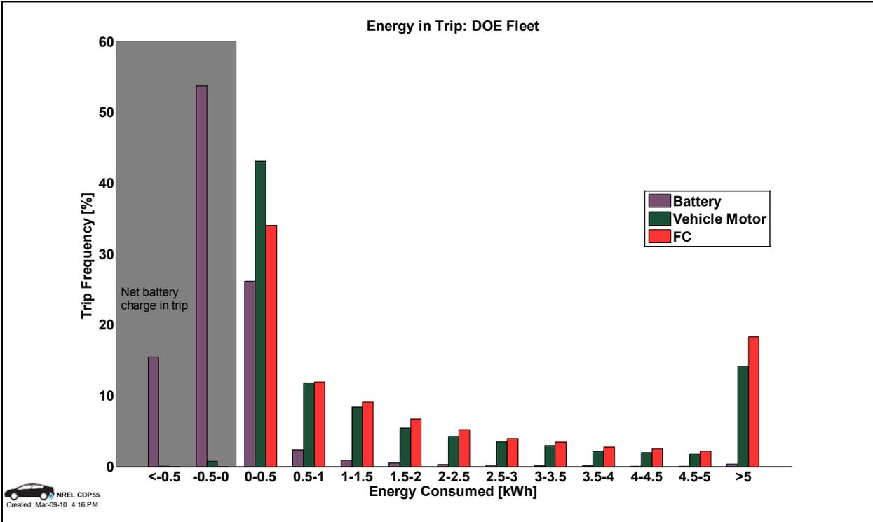
Figure 20: Fuel cell system energy in trips (CDP55)
