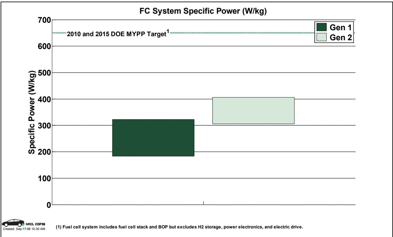
Figure 34: Fuel cell system specific power (CDP59)
