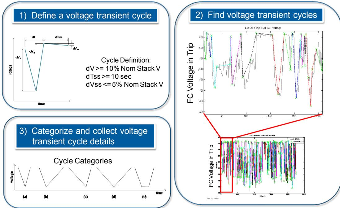
**Figure 12: Approach for characterizing voltage transient cycles**
