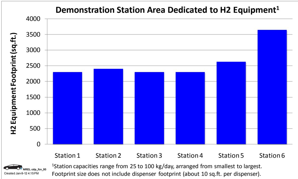
Figure 125: Demonstration hydrogen station equipment footprint (CDP93)
