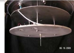
Antenna (4" monopole) mounted to baffle plate on tank lid
