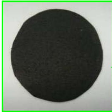
Activated carbon cathode works almost as well as Pt catalyst
