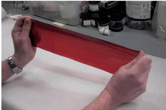
Figure 5-6: PBI sol-gel membrane
