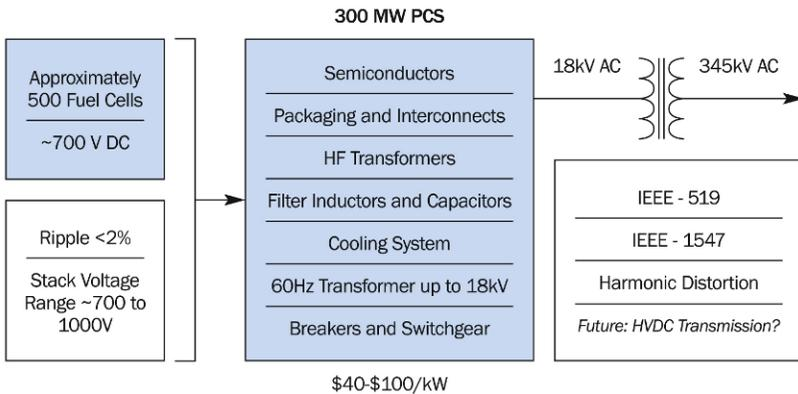
Figure 7-6: FC power plant requirements for high-megawatt PCS
