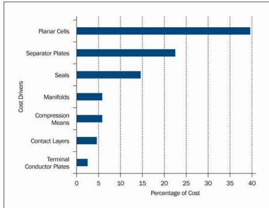
Figure 4-4: Cost drivers for planar ceramic fuel cells
