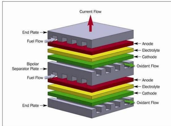
Figure 6-1: Schematic of repeat unit in a planar SOFC stack
