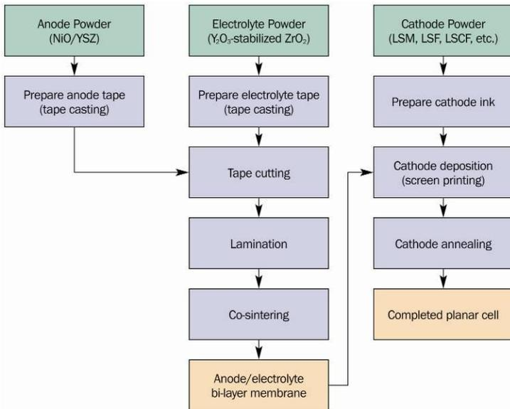
**Figure 6-5: Fabrication of anode-supported planar cells by co-sintering of anode and electrolyte layers, followed by deposition of cathode layers**
