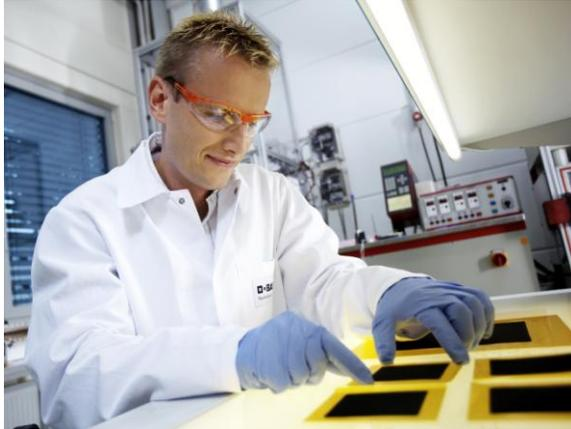
Figure 5-5: High temperature PEM MEAs
