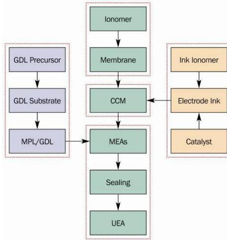
Figure 5-2: Low temperature polymer CCM
