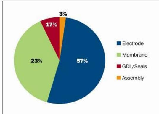
Figure 5-4: Current Cost Breakdown for LT MEA
