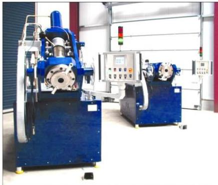
**Figure 6-18: Extrusion equipment for small diameter, anode substrate tubes**
