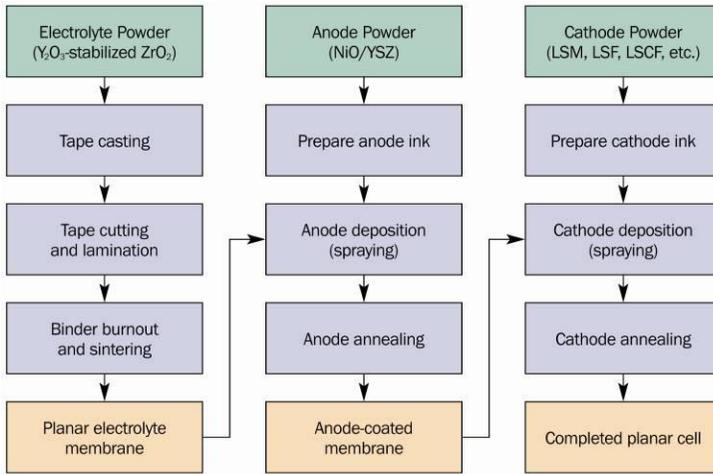
Figure 6-6: Fabrication of electrolyte supported planar cells by fabrication of electrolyte membranes, followed by separate deposition steps for anode and cathode layers
