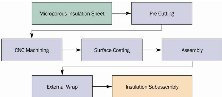
Figure 6-25: Insulation process flow
