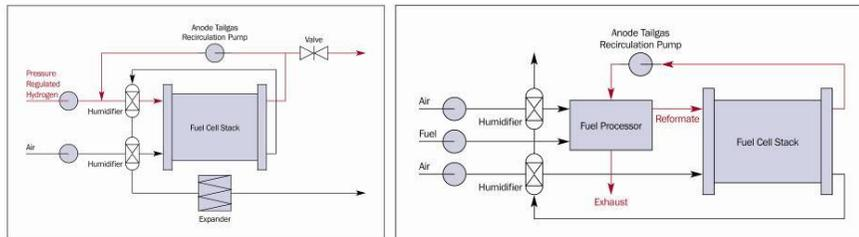
Figure 7-4: Simplified MHE and reformat fuel and oxygen delivery subsystem
