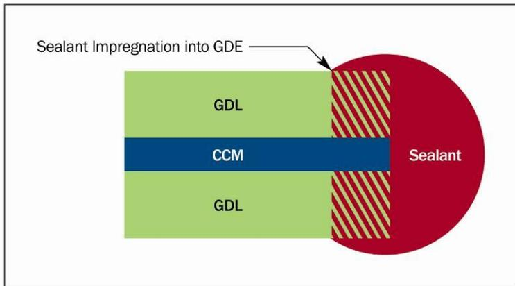
**Figure 5-16:** Edge-sealed (or flush-cut) MEA construction
