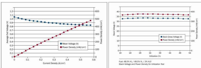
Figure 6-8: Sample performance curves, generated on as-built planar SOFC stacks
