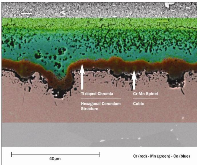
Figure 6-12: Ce-modified ( $Mn_{0.5}Co_{0.5}$ ) 304 spinel coatings on AISI 441 steel [6]
