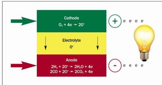
Figure 6-9: Electrochemistry of the SOFC; defines the gas environments and temperatures required for the materials of construction
