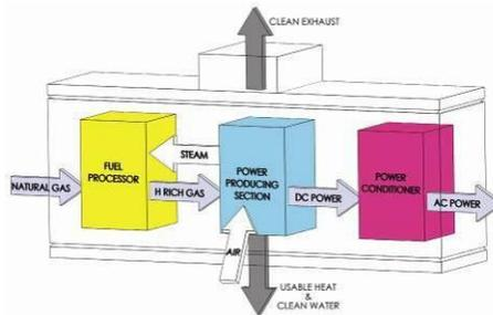
Figure 6-10: Block diagram of a fuel cell power system
