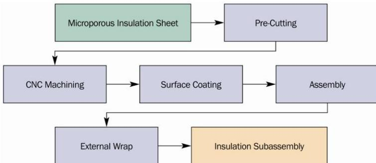
**Figure III-4: Process to insulate components using Microtherm® microporous sheets**
