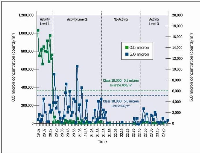
Figure 6-21: Particle level change in a clean room with different activities
