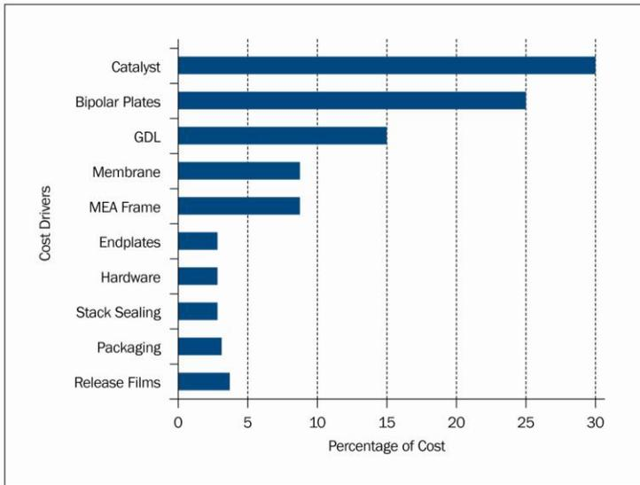
Figure 4-3: Cost drivers for polymer fuel cell stacks
