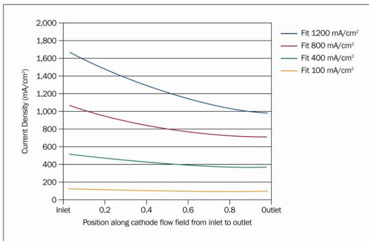
Figure III-3: Local current density along the flow field at different overall current densities
