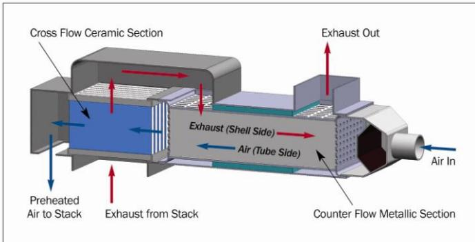
Figure 7-9: Ceramic/metallic heat exchanger system
