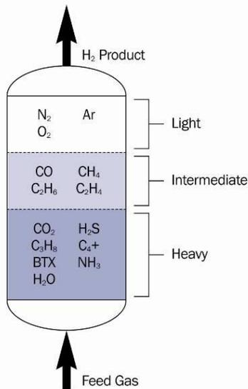
Figure 8-4: Schematic representation of PSA tank
