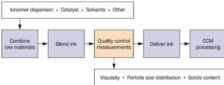
Figure 5-10: Current process for ink mixing and delivery
