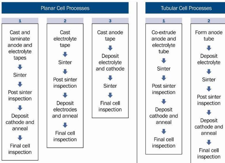
Figure 6-20: Process flow for planar and tubular ceramic cell manufacturing
