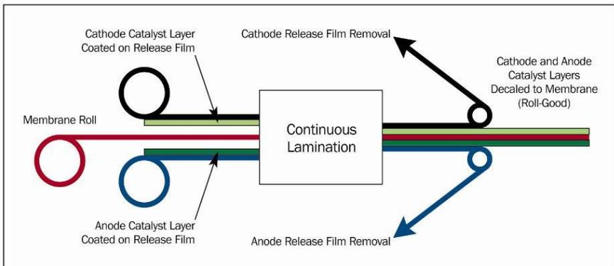
Figure 5-12: Schematic of continuous lamination
