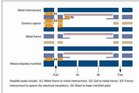
Figure 6-14: Possible seal types in a planar SOFC stack [4]
