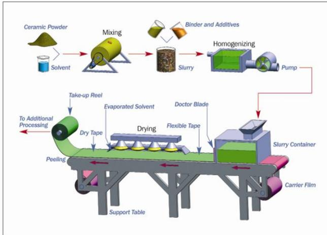
Figure 6-3: Schematic of tape casting process for making green tape layers
