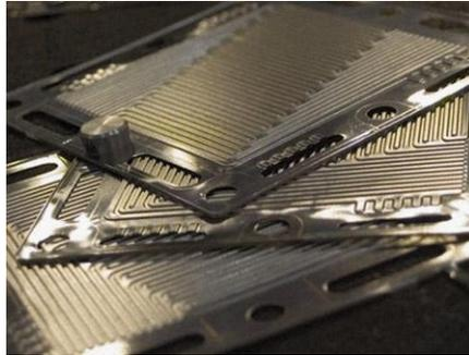
Figure 5-20: Example of Metal Bipolar Plates
