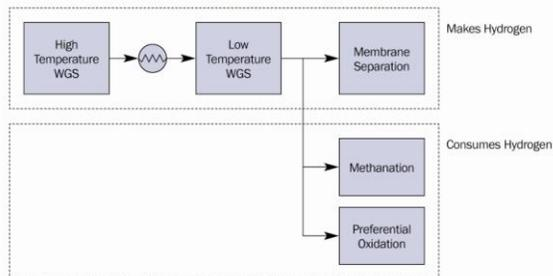
Figure 8-3: Schematic of carbon monoxide cleanup process
