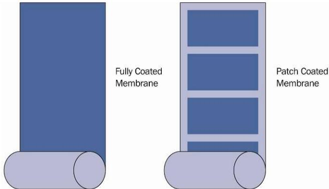
Figure 5-14: Comparison of fully coated and patch coated membrane
