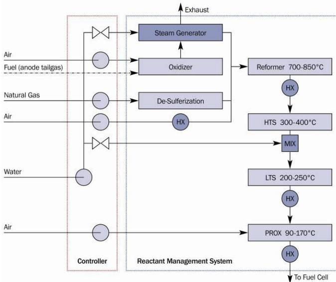
Figure 7-3: Gaseous flow through the RMS
