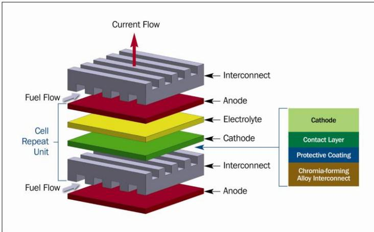
Figure 6-11: Technical focus for interconnect materials and coatings gap resolution [5]
