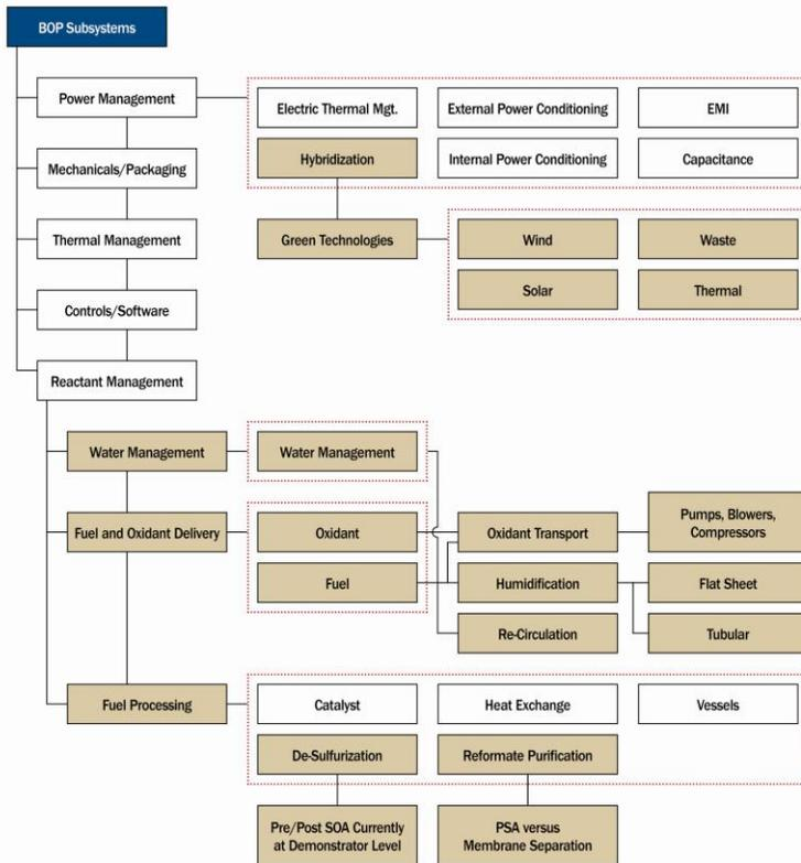
Figure 7-2: Focus area breakdown for balance of plant
