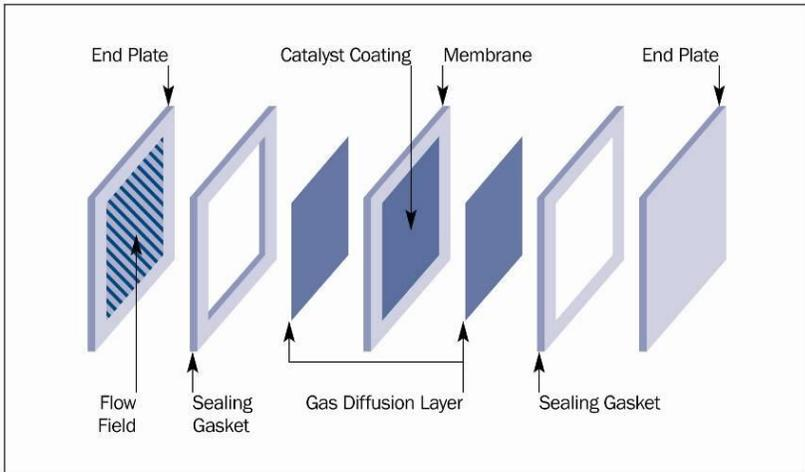
Figure 5-1: Elements of a typical Unitized Electrode Assembly (UEA)
