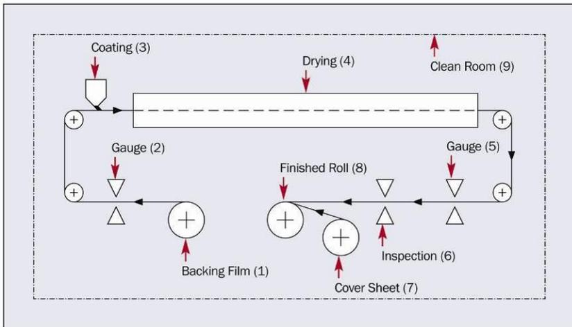
Figure 5-7: Thinner membrane manufacturing processes
