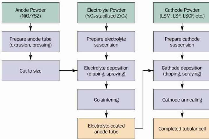
Figure 6-17: Isostatic pressing of anode supported tubular cells
