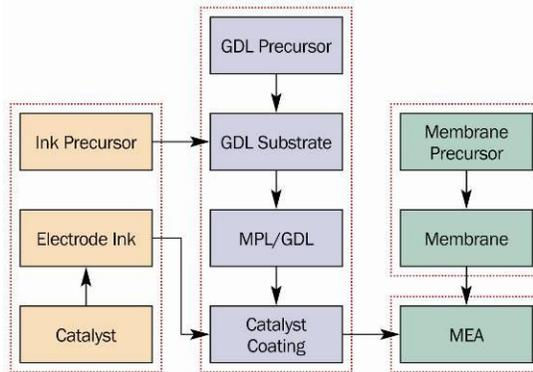
Figure 5-3: High temperature PBI-based MEA
