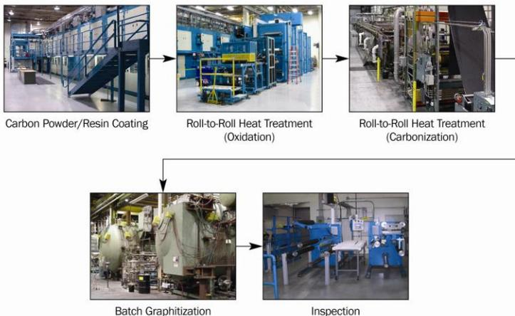
**Figure 5-8: GDL manufacture involves multiple processing steps**
