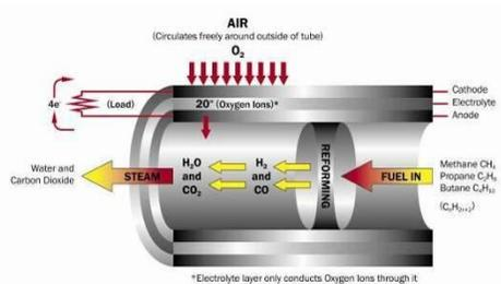
Figure 6-2: Schematics of tubular solid oxide fuel cell stacks
