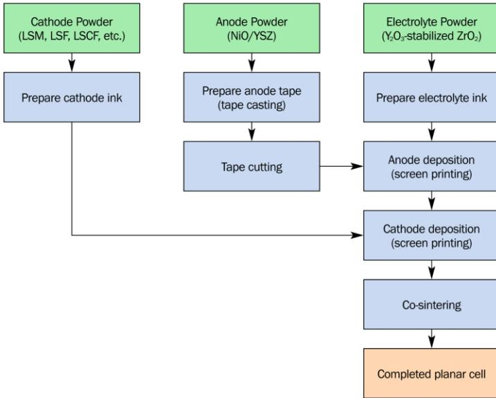
**Figure 6-4: Fabrication of anode-supported planar cells by co-sintering of anode, electrolyte, and cathode layers**
