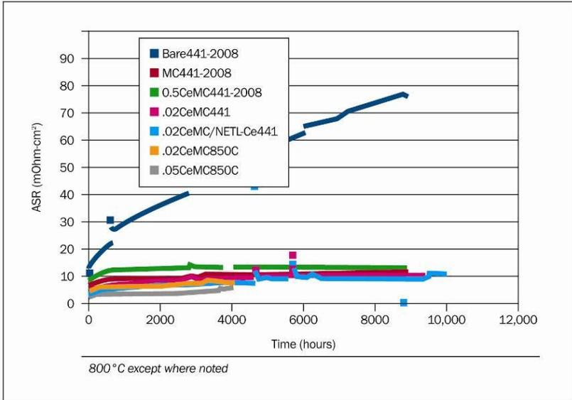
**Figure 6-13: Long-term area specific resistance (ASR) measurements: 800 °C and 850 °C [6]**
