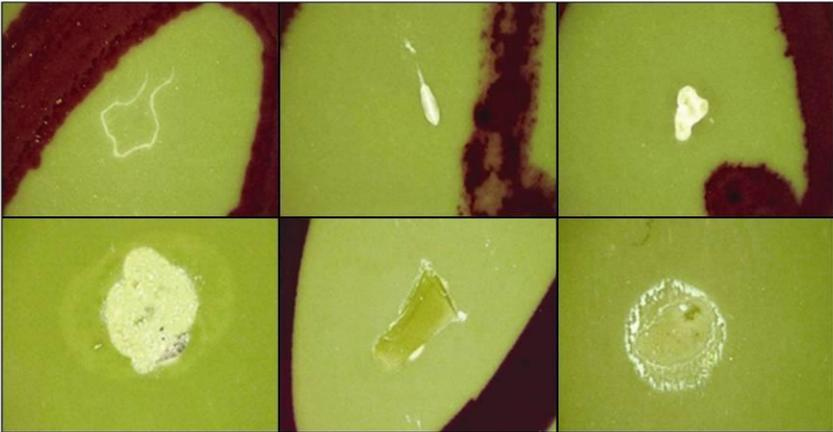
Figure 6-22: Flaws found in the post-sintering inspection of fuel cell components
