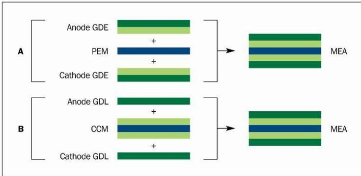
Figure 5-11: Membrane electrode assembly (MEA): A- GDE-based; B- CCM-based
