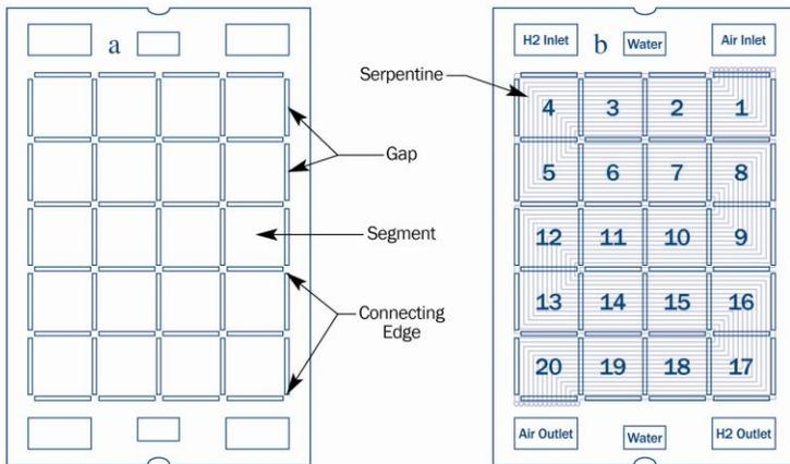
Figure III-2: Numbering the flow field measurement points on the cathode side
