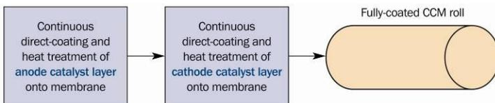
Figure 5-13: Schematic of a direct-coated process
