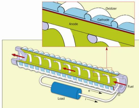
Figure 6-19: Current collectors along the exterior and interior of the SOFC MEA [8]
