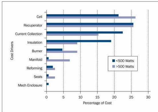
Figure 4-5: Cost drivers for tubular ceramic fuel cells
