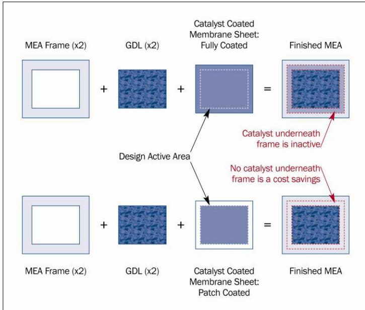
Figure III-1: Schematic of patch coating methods
