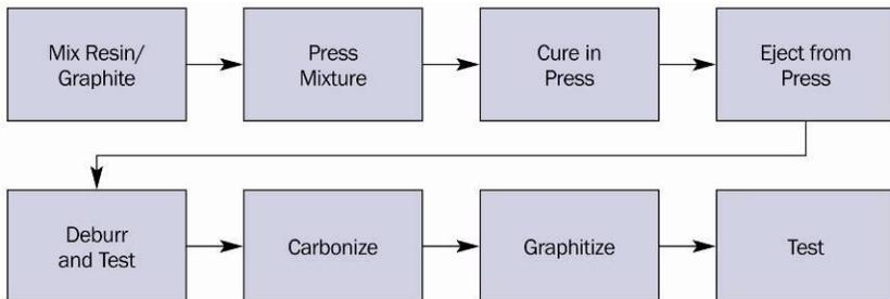
Figure 5-19: HTPEM bipolar plate compression process
