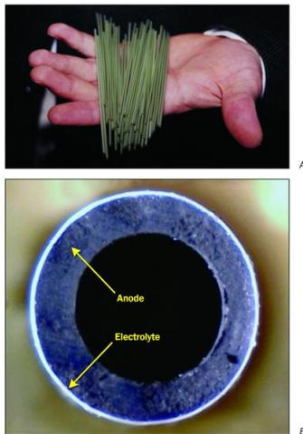
**Figure 6-16: Anode-supported micro-tubular elements (prior to cathode deposition)**
