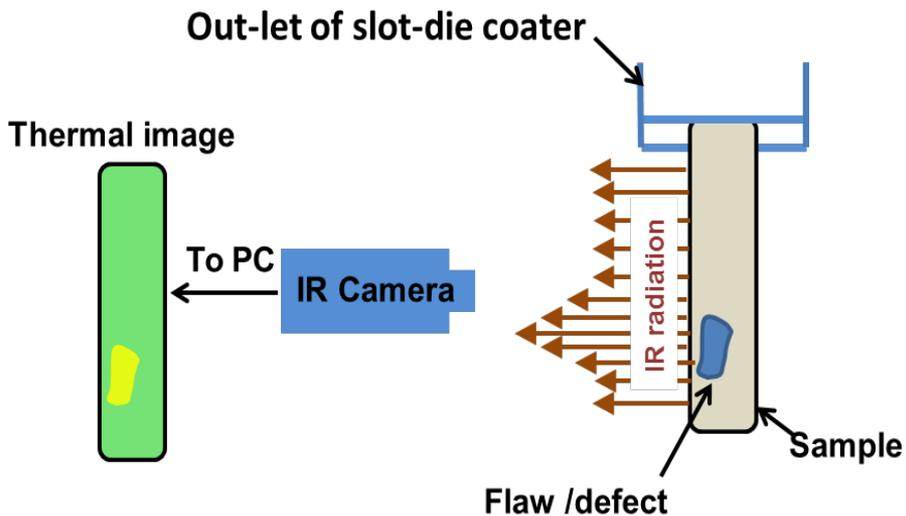
**Schematic of IR thermography method to detect flaws in dry electrodes**
